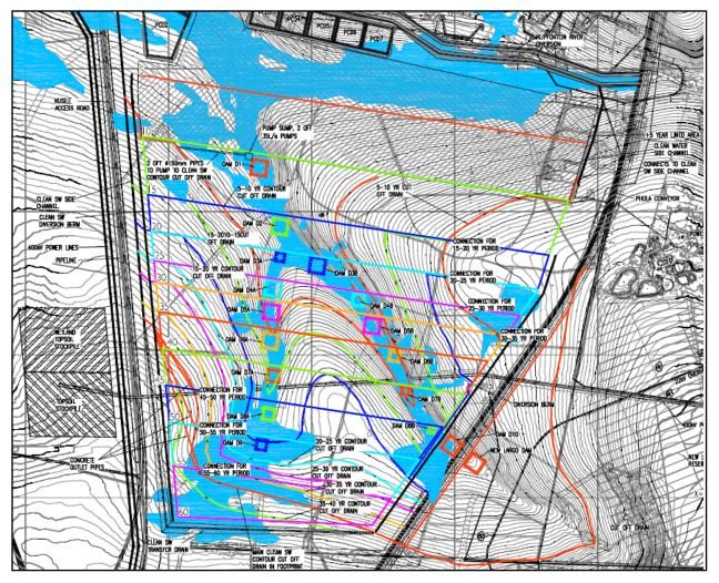
Figure 11: Layout of Clean Storm Water Dams and Pollution Control Dams
