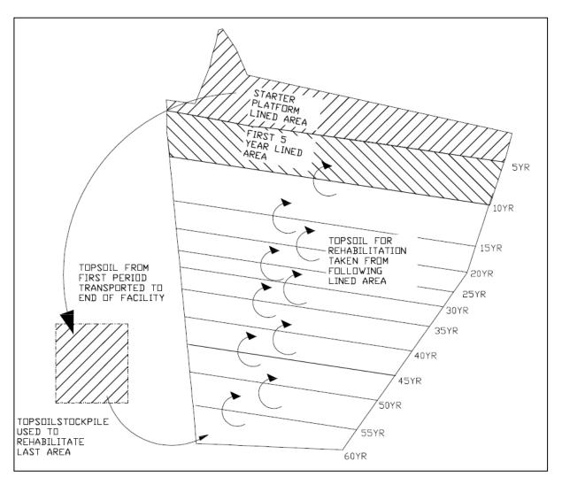
Figure 14: Method of progressive topsoil management
