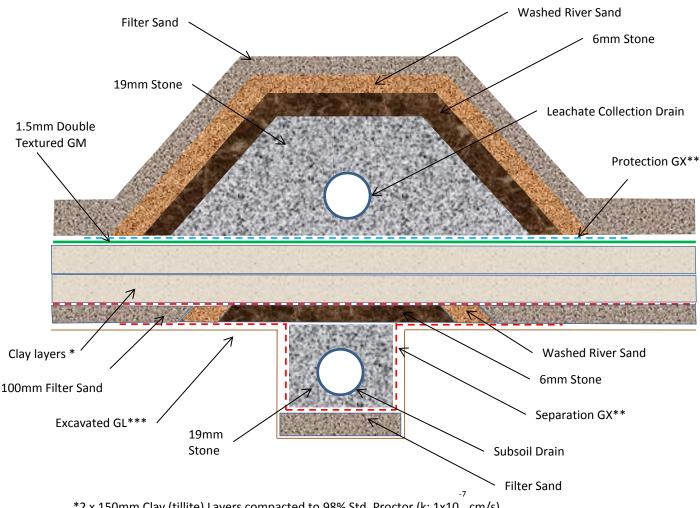
\*2 x 150mm Clay (tillite) Layers compacted to 98% Std. Proctor (k: 1x10 cm/s). \*\*GX = Geotextile \*\*\*GL = Ground Level
