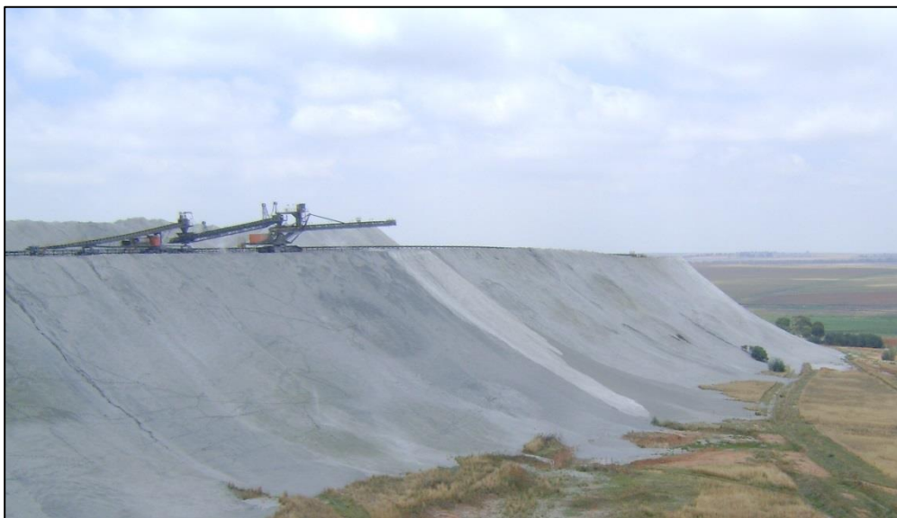
Figure 4: Typical stacking ash at angle of repose (as seen at Kendal Power Station)
