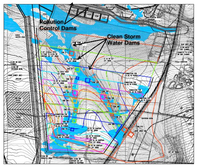
Figure 8-9: Layout of Clean Storm Water Dams and Pollution Control Dams
