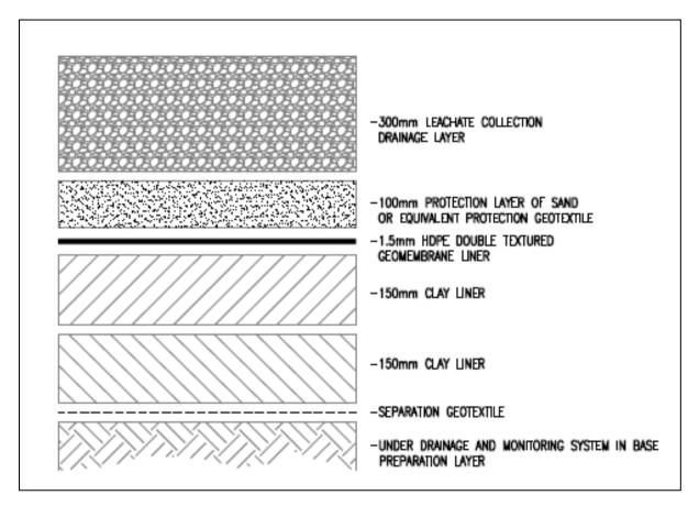
Figure 8-4: Class C Liner Specification in terms of DEA Norms and Standards
