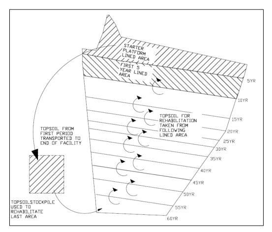
Figure 8-10: Method of progressive topsoil management
