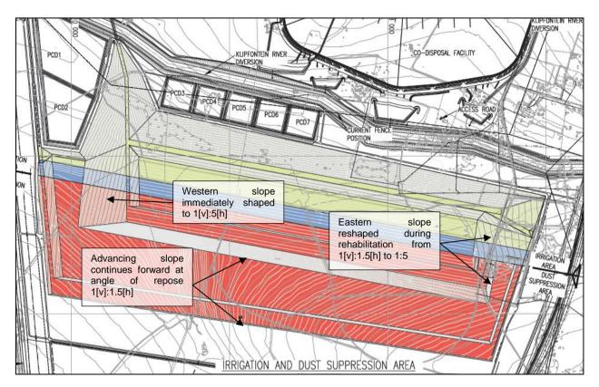
Figure 9-3: Reshaping on eastern side of facility
