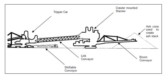
Figure 8-7: Stacker setup
