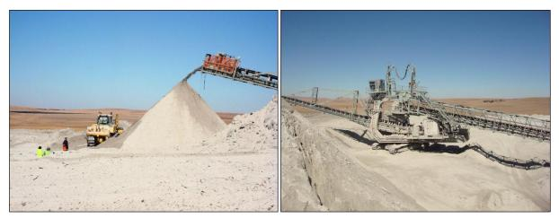
Figure 4.4: Stacker being used to dispose of ash at the Majuba Power Station
