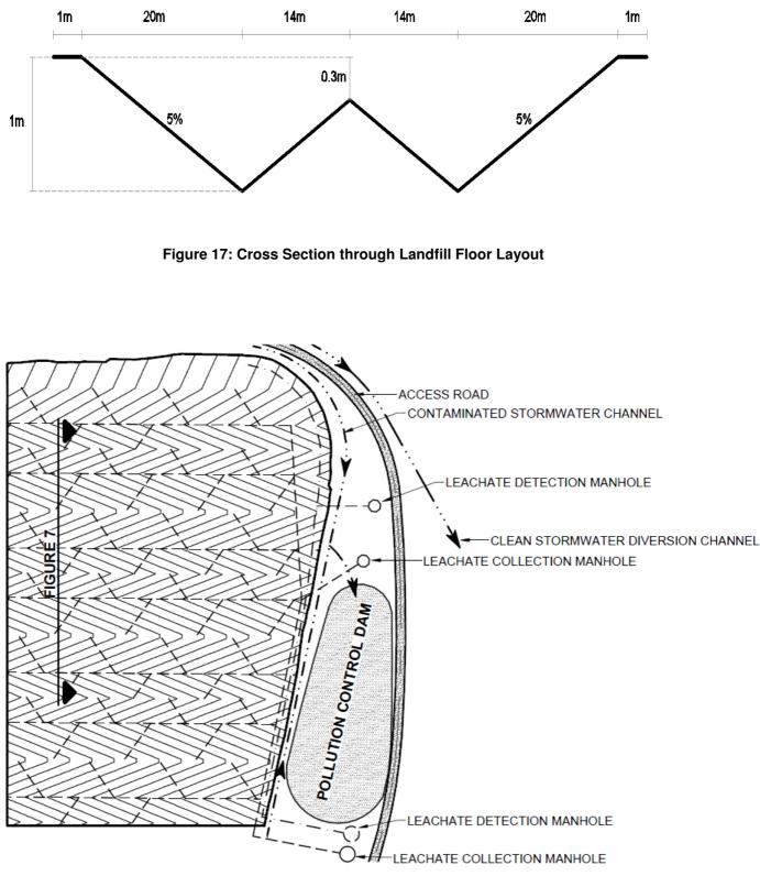
Figure 18: Herringbone Arrangement of Leachate Collection Pipes
