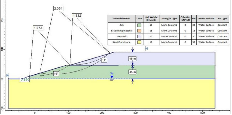
Figure 5 – Circular Slip Failure with a slope gradient of 1V:3H (Piggy-backing Scenario)
