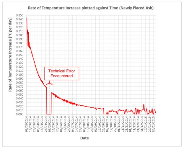
Figure 7 - Rate of Temperature Increase for the newly placed ash pile
