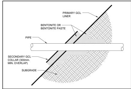
Figure 3: Typical pipe penetration section detail (after ASTM D 6102) (Note: change min overlap to 500mm)
