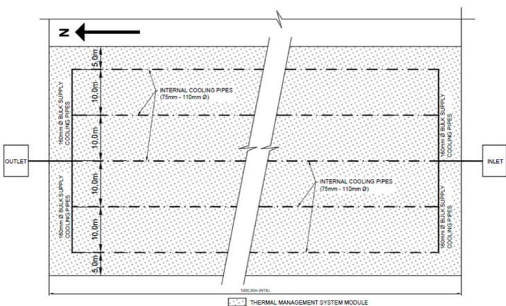
Figure 12 - Proposed thermal management system module for ADF waste cells
