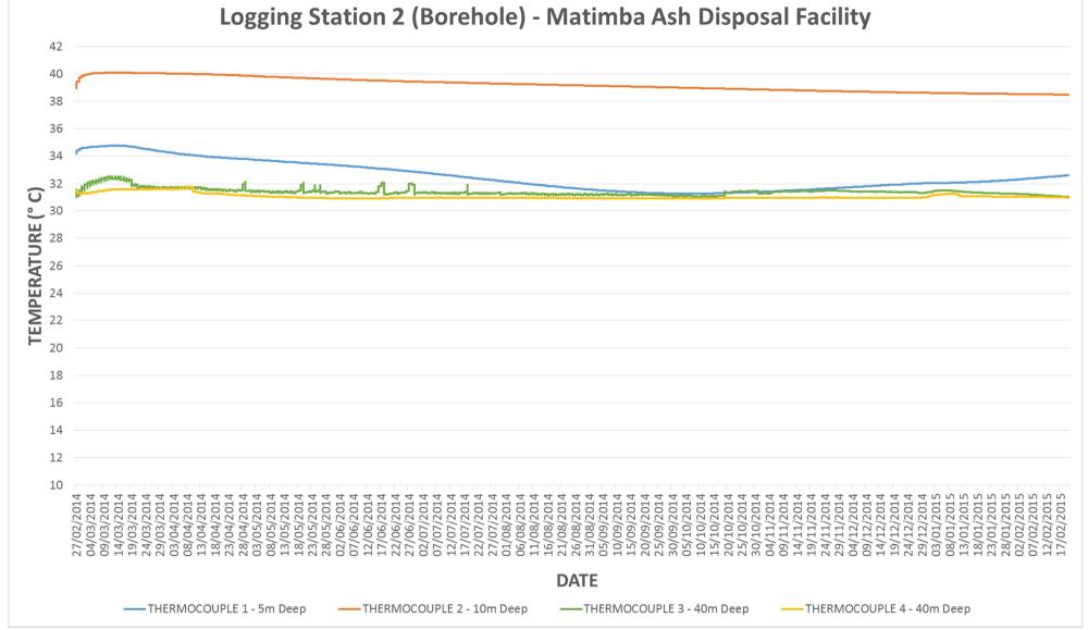
Figure 8 - Temperatures recorded at Logging Station 2 (Borehole 2) from April 2014 to February 2015
