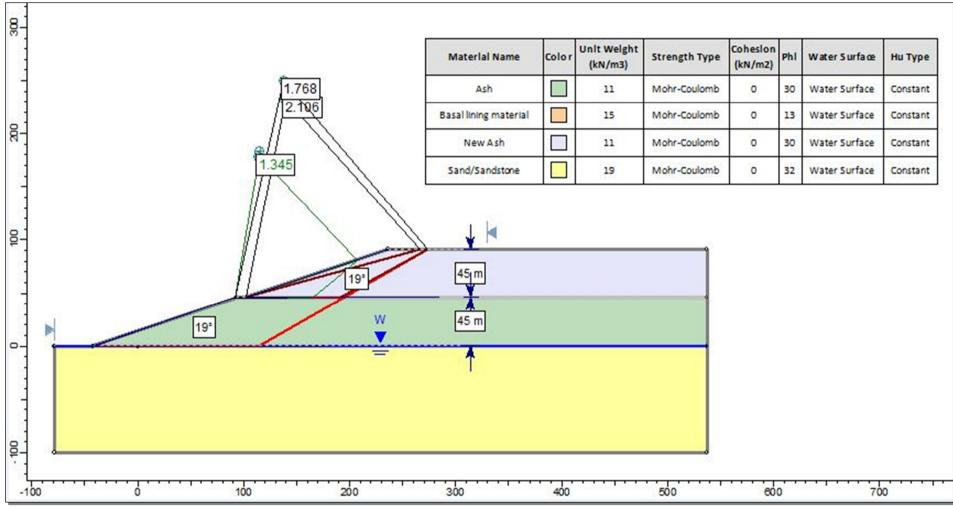
Figure 4 - Block Failure with a slope gradient of 1V:3H (Piggy-backing Scenario)
