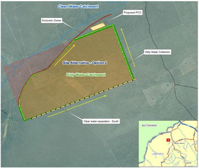
Figure 2: Site Alternative 2-Recommended Storm water Management Measures (GCS,2013)
