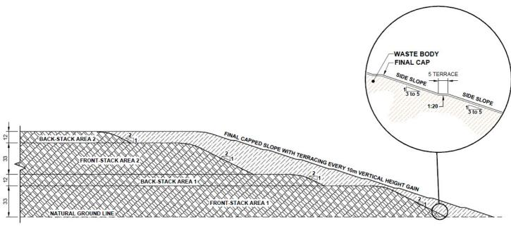
Figure 20: Ash Landfill Development and Final Capping
