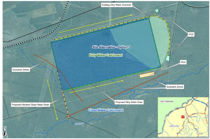
Figure 1: Site Alternative 1-Recommended Storm water Management Measures (GCS,2013)
