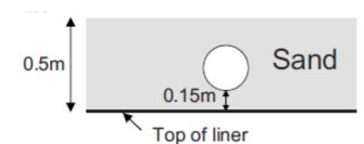
Figure 10 - Location of the cooling pipes taken from Rowe et al. (2010)
