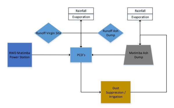
Figure 11.1: Process water flow diagram of the existing Matimba Ash disposal facility
