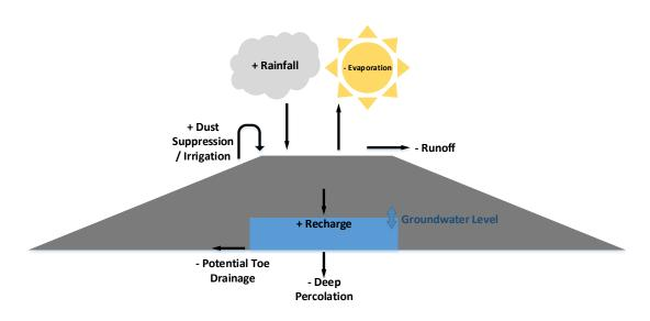
Figure 11.2: Schematic Ash Pile Water Balance
