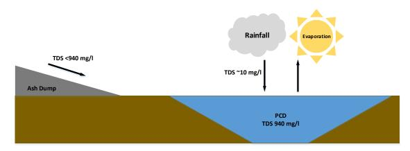
Figure 11.5: Schematic overview of a PCD Salt Balance
