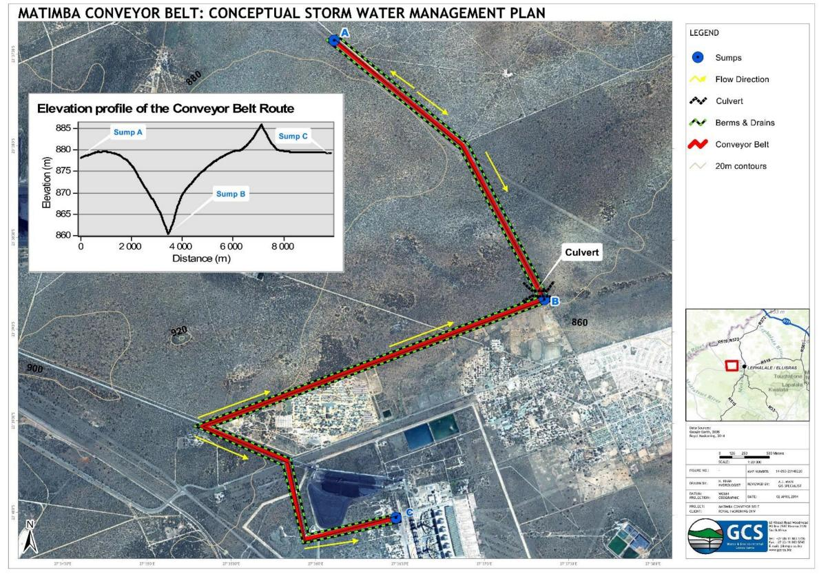
Figure 10.5: Conceptual Storm Water Management Plan for the Matimba Conveyor Belt
