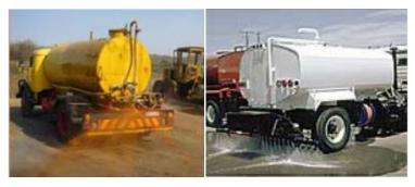
FIGURE 20: EXAMPLES OF WATER SPRAY EQUIPMENT
