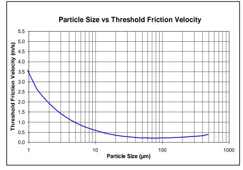
FIGURE 17: PARTICLE SIZE CURVE FOR WIND EROSION CALCULATIONS
