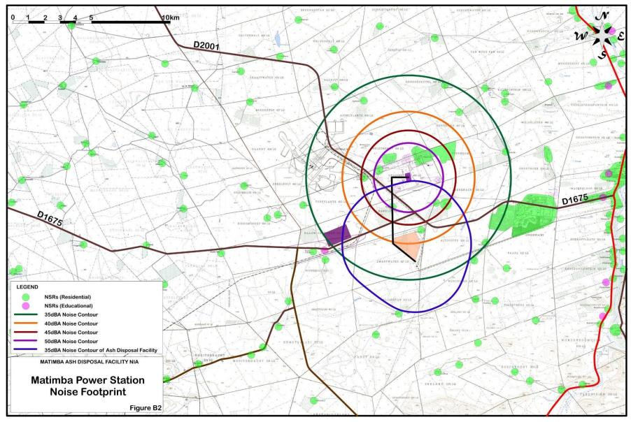
Figure B2: Matimba Power Station Noise Footprint
