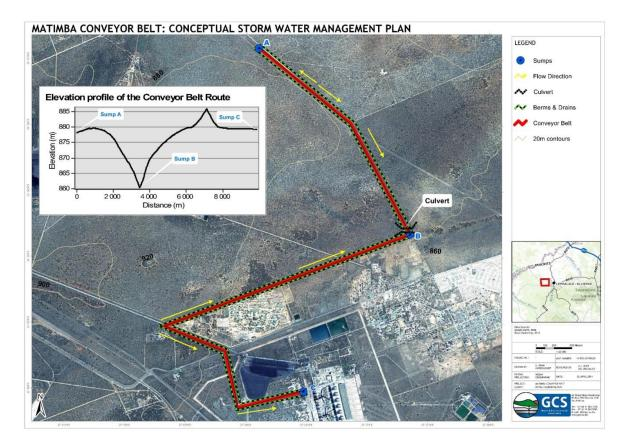
Figure 44: Conceptual stormwater management plan for the linear infrastructure route
