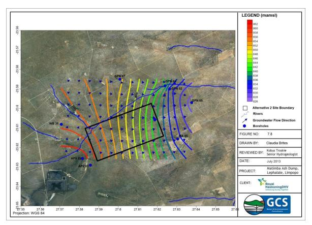
Figure 34: Site Alternative 2 groundwater flow direction
