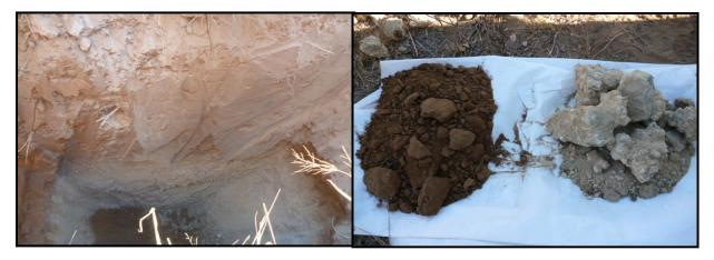
Figure 18: Aeolian sandy soils underlain by calcrete (left) and colluvial soils and nodular calcrete (right)
