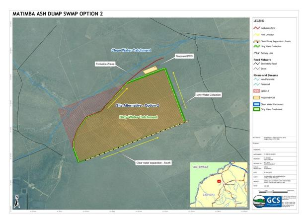
Figure 42: Site Alternative 2 conceptual stormwater management measures
