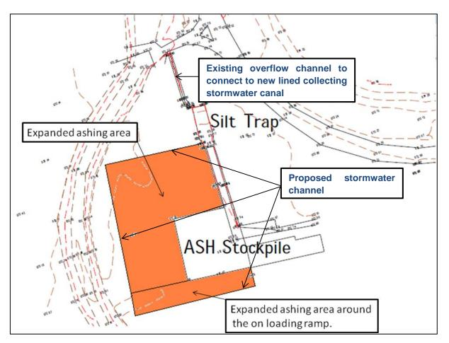
Figure 6: Proposed expansion and stormwater management of the emergency ash offloading area
