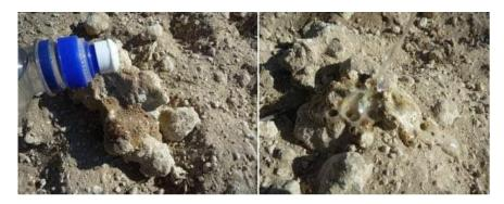
Figure 66: Addition of HCI (10 % solution) to subsoil lime and effervescence confirming the presence of carbonates
