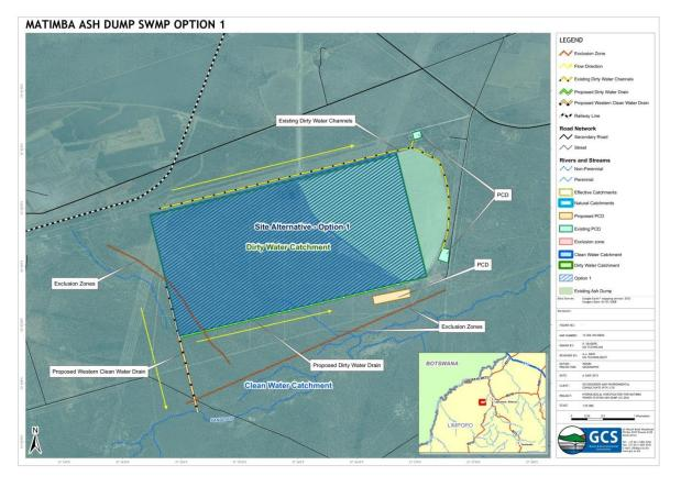
Figure 41: Site Alternative 1 conceptual stormwater management measures
