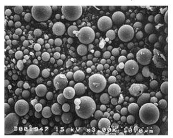
Figure 26: Ash particle magnified x2000
