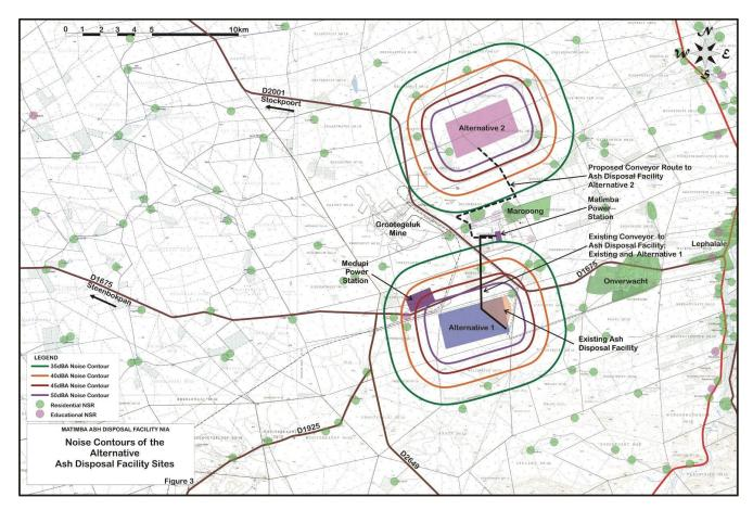
Figure 87: Noise contours of the ADF site alternatives
