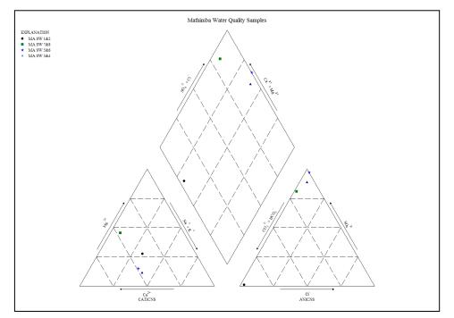
Figure 40: Piper diagram for surface water samples
