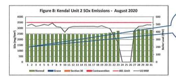
Note that gaseous emissions for unit 2 were manually entered using Independant third party QAL2 parallel test reports due to defective CEMS monitors, but unit 2 CEMS monitors startd working from the 21st of August 2020 after repairs
