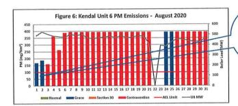
Unit 6 high PM emissions can be attributed Precipitator conveyor 23 that kept tripping, 503 plant was on hold mode due to sulphur flow low, 503 plant was off due to sulphur plant atteam isolated to remove blocked who end steam temperature low and Dust Handiling Phant tripping due to full compartments
