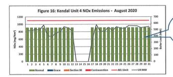
Note that gaseous emissions for unit 4 were manually entered using Independant third party QAL2 parallel test reports due to defective CEMS monitors.
