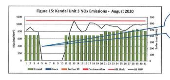
Note that gaseous emissions for unit 3 were manually entered using Independant third party QAL2 parallel test reports due to defective CEMS monitors.
