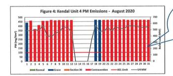
Unit 4 high PM emissions can be attributed to SO3 paint off for steam pipe and converter steam leok repoils and dust handling plant was off due to comportment levels full. Precipitator conveyor 22 was not running, comportment 30 knile gates were light and 30 spindle was broken
