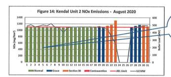
Note that gaseous emissions for unit 2 were manually entered using Independant third party QAL2 parallel test reports due to defective CEMS monitors.
