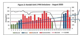
Unit 2 high PM emissions can be attributed to 503 plant tripping due to back end temperatures low and Dust Handling plant tripping due to high compartment level
