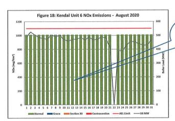
Note that gaseous emissions for unit 6 were manually entered using Independant third party QAL2 parallel test reports due to defective CEMS monitors.
