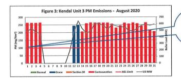
Unit 3 high PM emissions can be attributed to compartment levels high and knije gates closed, streams not available and top bunker conveyor kept tripping
