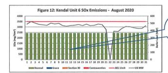
Note that gaseous emissions for unit 6 were manually entered using Independant third party QAL2 parallel test reports due to defective CEMS monitors.
