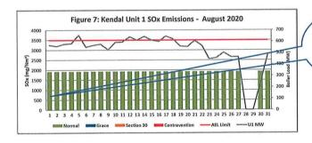
Note that gaseous emissions for unis 1 were manually entered using independant third party QAL2 parallel test reports due to defective CEMS monitors.
