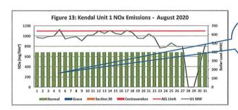
Note that gaseous emissions for unit 1 were manually entered using Independant third party QAL2 parallel test reports due to defective CEMS monitors.
