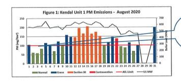
Unit 1 high PM emissions can be attributed: 1.503 plant that frequently tripped due to defective dilution air control volvie from the 1st to 18th of Jugust. 2.Dust Handling plant tripping due to high compartment level from the 20th August.
