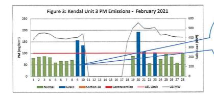
Unit 3 high PM emissions on the 9th-10th was due to unit trip on the 9th and was synchronised on the same day. Unit 3 high PM emissions on 20,21& 23 can be attributed to six ESP fields and precipitator chain conveyor 21 tripping, high back end temperatures and to low Fuel Factor.
