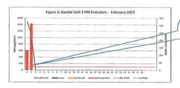
High PM emissions can be attributed to The high PM emissions can be attributed to stream 2 stopped due to second collecting conveyor plumber dock that was damaged. Peedp conveyor 22, 24 kept on tripping. SO3 plant on hold due to steam temp low. Peedpt 24 fast to start due to ash accumulation on the sprocket.
