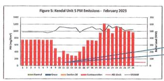
High FAI emissions can be attributed to High FM emissions can be attributed to The High FM emissions can be attributed to streem 2 stopped due to second collecting conveyor pumber clack that was damaged. Presig conveyor 72, 24 kept an tripping, SOJ plant on half due to steem temp law. Precipt 24 fills to start due to all convenients on the spreader.
