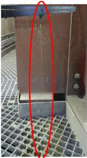
Figure 5: 151m Platform Beam – Draw-wire to Measure Deflection
