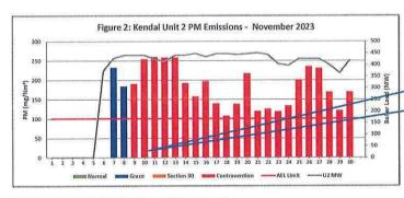
High emissions can be attributed to Precip fields 11, 12, 22 and 44 of fan faulty, Field 11 no internals, Field 13,14,15 indicating internal short circuit, F44 has electrical faults - Fan failure. Stream 2, 1st collector O/C, communication fault on the system from Unit 1-6, High back end temps pcp13 choked and all knife gates shut, 5 precip fileds
