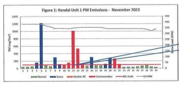
High emissions can be attributed to SO3 plant not running due to low Sulphur flow. SO3 pipe line blocked. PCP 13 triped all knile gates are closed due to compartments high levsly, filled performance deteriorating, F24 – Fan failture, unit had ashbacklogs.
