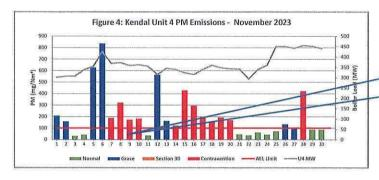
High Photenissions can be attributed to THS an pcp 12-19 standing with all knife gates shut, faulty on first collection stream 1, pcp 11-14 all knife gates closed (stream 1 tripped) gailty on first collection stream 1. Stream 12 ad collector not available, LH draught group was shud down, Stream 21st collector gearbox mechanically defective, first collector stream 1 kept tripping, Stream 1 First Collector checked (PCP 11-14 OFF and all Knife gates closed) bucket elevator blackage
