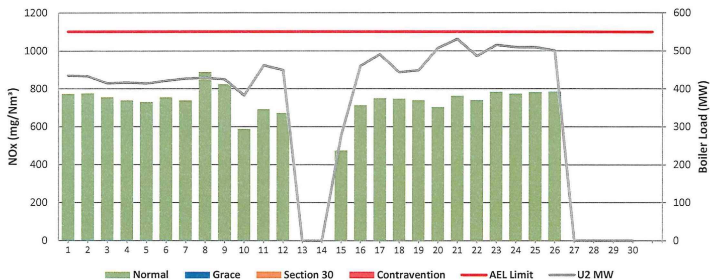
Figure 12: Duvha Unit 2 NO x Emissions - September 2024
