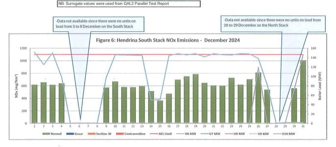
Gaseous Emission Trends (NOx and SOx) for the North Stack: Surrogate values from QAL2 Parallel Test Report (RSL 411) have been used due to erronous data from the Continuous Emission Monitoring System (CEMS). Spot Check measurements have been performed internally and they confirm the error.
