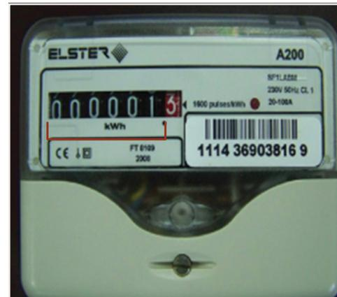
Figure 7: Elster kWh meter with 6 numbers. All 6 of the numbers to the left of the comma must be read including any zeros. This reading would be 000001
