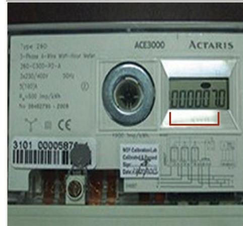
Figure 3: Actaris kWh meter with 6 numbers and one decimal. Read the first six numbers only, do not read the far right number after the comma. This reading would be 000007
