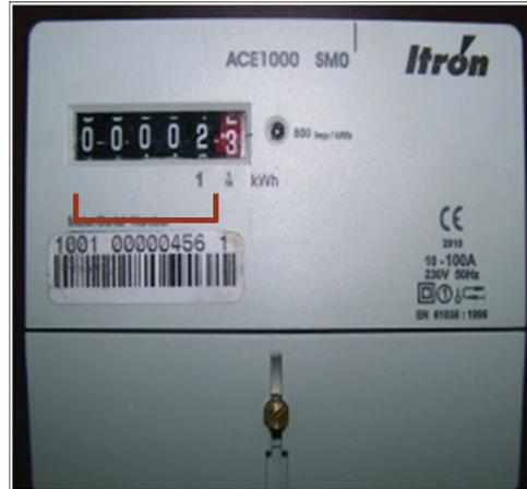
Figure 2: Itron kWh meter with 5 numbers. All 5 of the numbers must be read including any zeros before the comma. This reading would be 00002
