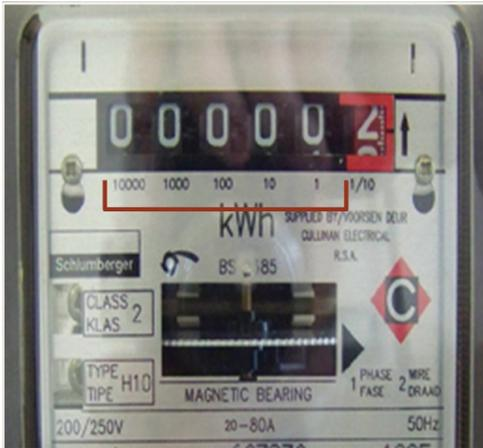
Figure 1: The Schlumberger kWh meter with 5 numbers. All 5 of the numbers up to the comma must be read, including any zeros. This reading would be 00000
