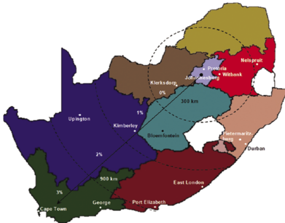
Figure 3: Transmission zones for loads
