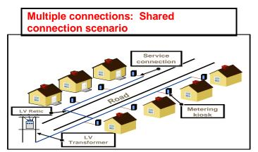
Multiple connections is where an LV reticulation network is supplying multiple customers and only the service cable is dedicated.
