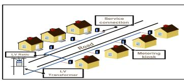
Multiple connections is where an LV reticulation network is supplying multiple customers and only the service cable is dedicated.
