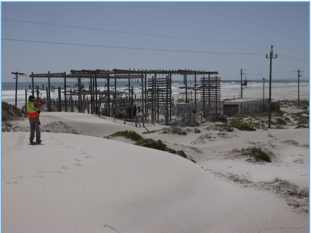
Frontispiece. The existing Insulator Pollution Test Station on the coast south of Koeberg, being swamped with wind-blown sand.
