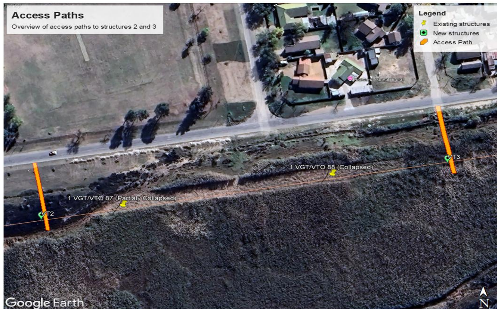
Figure 9: Proposed locations of construction access paths to be created
