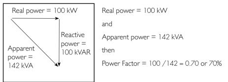
This indicates that only 70% of the power provided by the electrical utility is being used to produce useful work.
