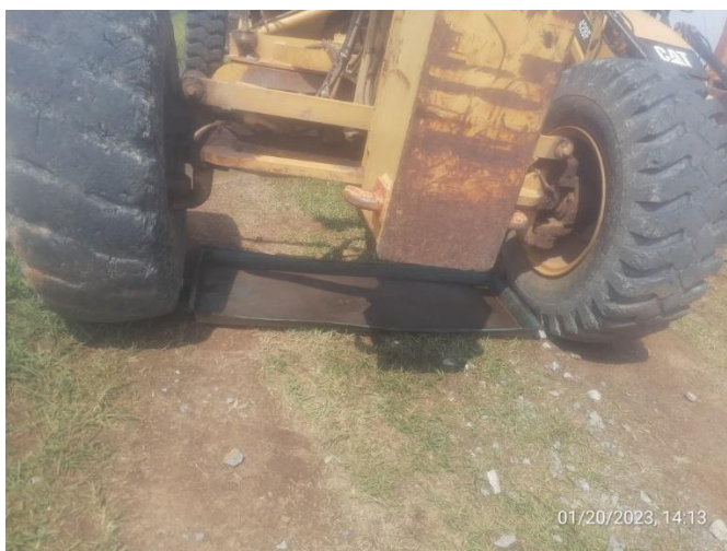
Figure 2: All stationary vehicles had drip trays underneath to prevent soil and groundwater contamination.
