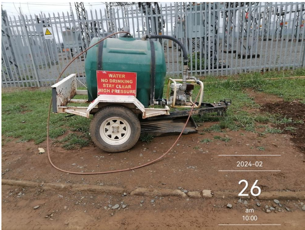
Figure 10: Water Bowser labeled with drip trays properly secured
