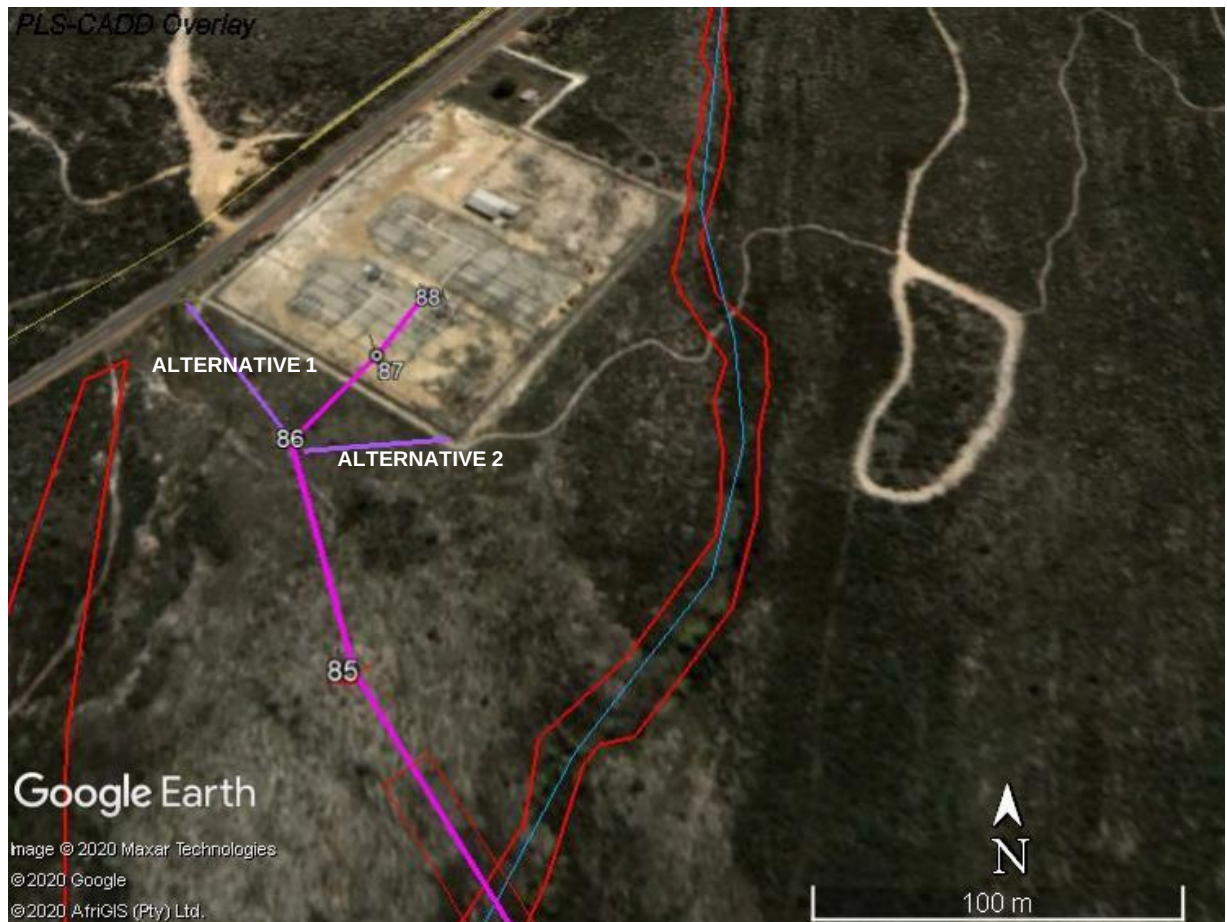
Figure 2.2 Alignment alternatives for a turning circle at the Witzenberg substation, to allow truck turning at proposed support structure 86.
