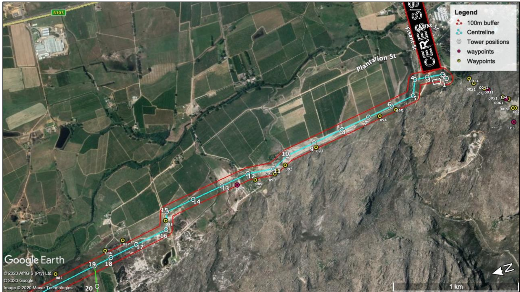
Figure 7.8.7. SURVEY MAP: Google Earth™ aerial image showing 100m corridor (red lines) and the proposed 132kV powerline (blue line), survey waypoints (yellow and pink numbered circle icons) and Towers 20 to Tower 1. Note the position of the north arrow on the rotated image.
