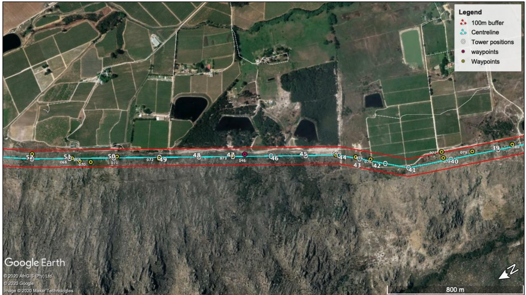
Figure 7.8.1. SURVEY MAP: Google Earth™ aerial image showing 100m corridor (red lines) and the proposed 132kV powerline (blue line) and Towers 52 to Tower 39 along the main powerline. Note the position of the north arrow on the rotated image.
