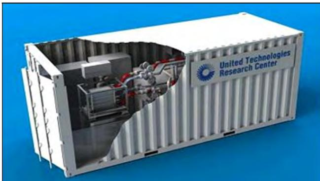
Figure 7: Flow battery storage container
