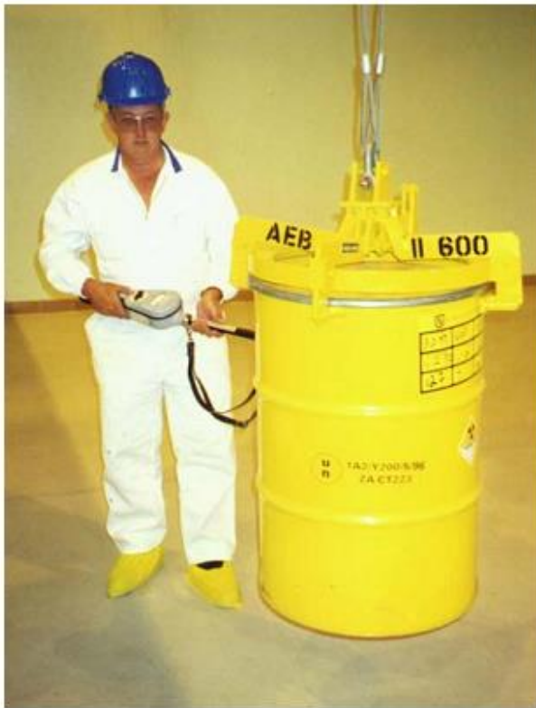
Figure 3-13: Standard steel and concrete containers used for radioactive waste disposal at Vaalputs
