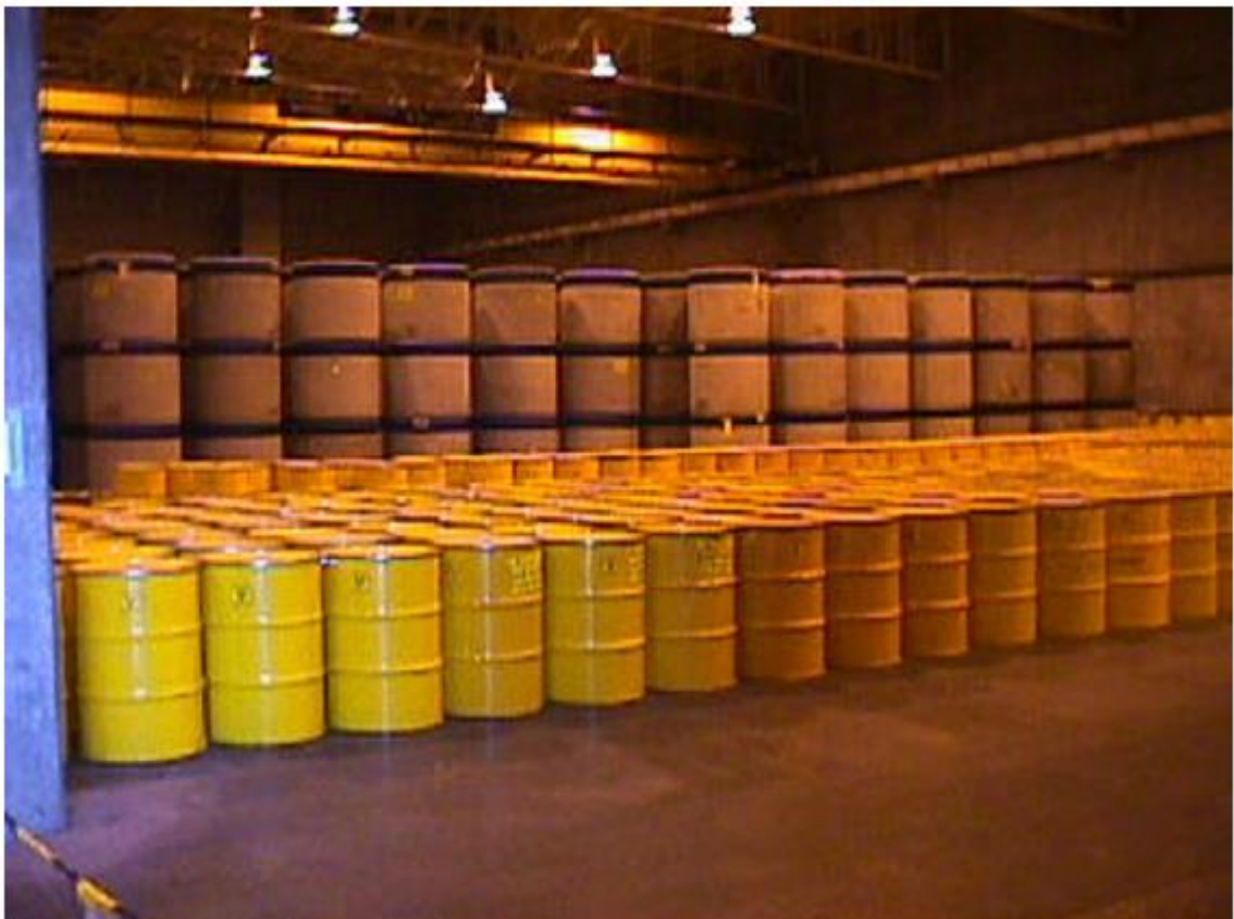
Figure 3-14: Storage facility for ILW and LLW showing concrete drums in the background and steel drums in the foreground
