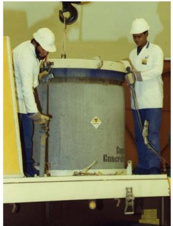
Figure 3-13: Standard steel and concrete containers used for radioactive waste disposal at Vaalputs
