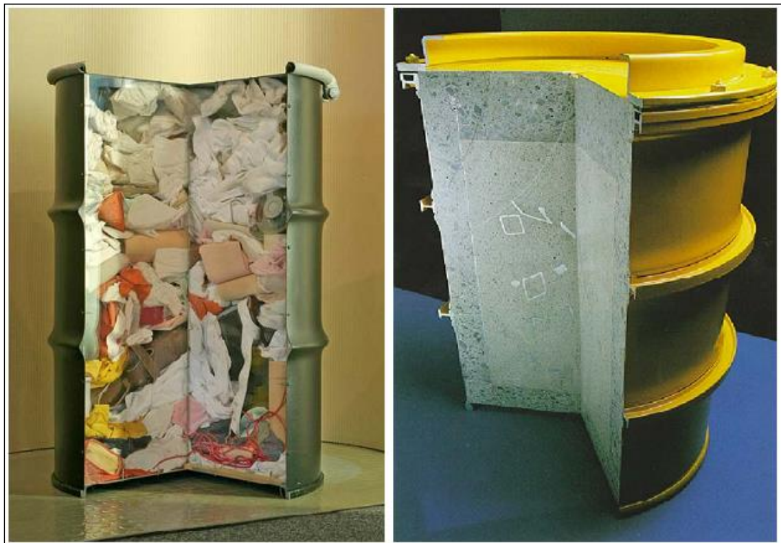
Figure 3-12: Compactable (LLW) and non-compactable (ILW) radioactive waste storage containers
