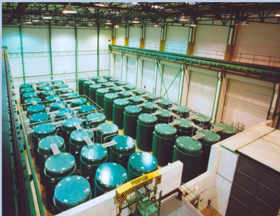
Figure 7-29: An example of a dry storage facility for spent nuclear fuel
