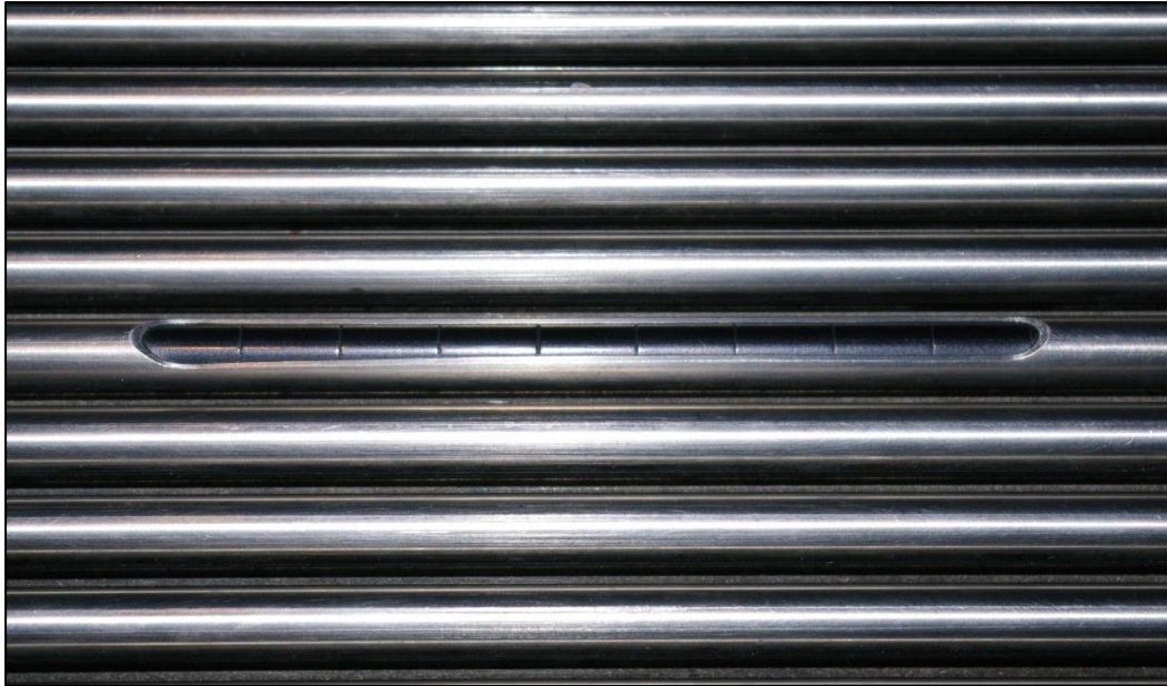
Figure 3-4: A display of nuclear fuel pellets in a cladding tube at Koeberg Nuclear Power Station
