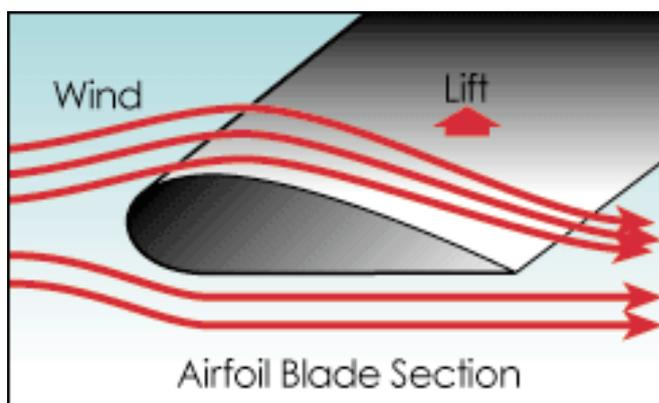
**Figure 3.5:** Illustration of the principle of lift
