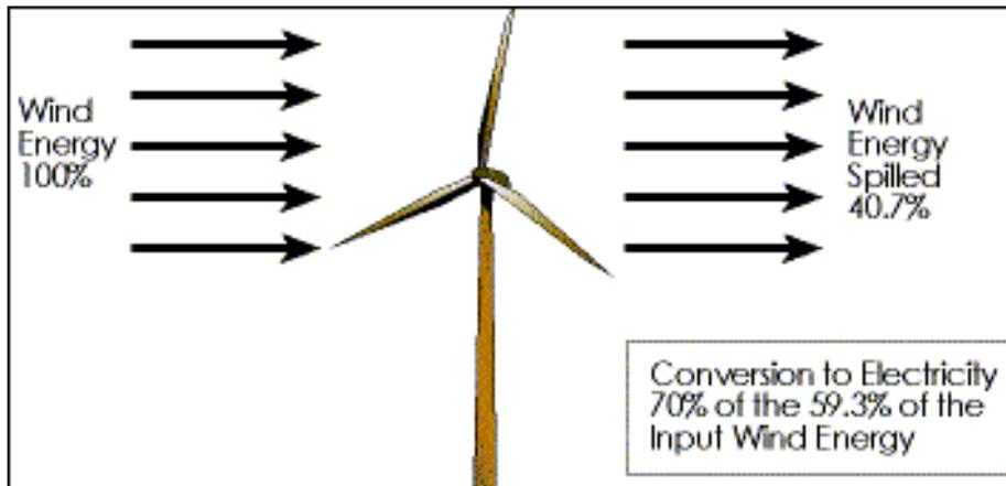
**Figure 3.7:** Illustration of the principle of the Betz Limit
