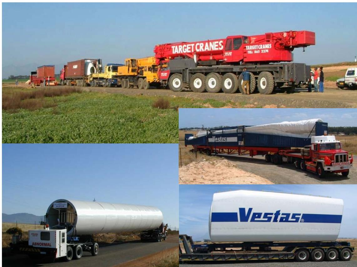
**Figure 7.2:** Photograph illustrating the equipment required for the transportation of turbine components to site (photographs courtesy of Eskom at during the construction of the Klipheuwel demonstration facility)
