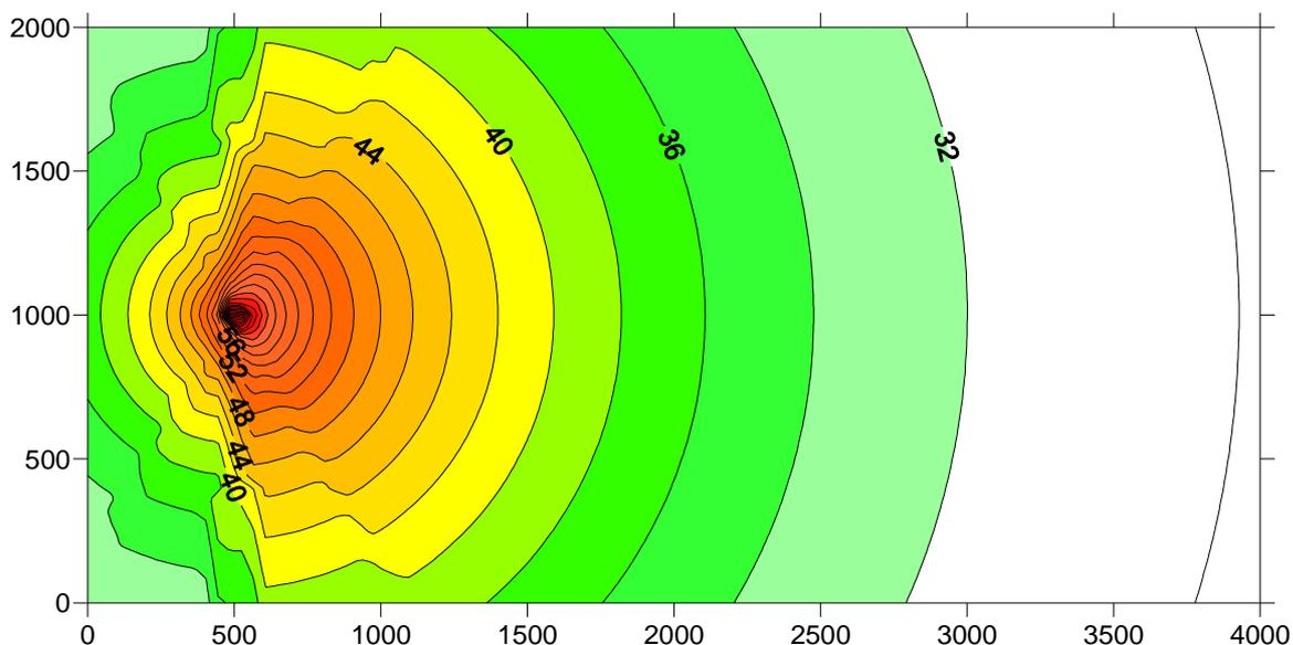
**Figure 6-1: One WTG operating, all hard ground scenario**
