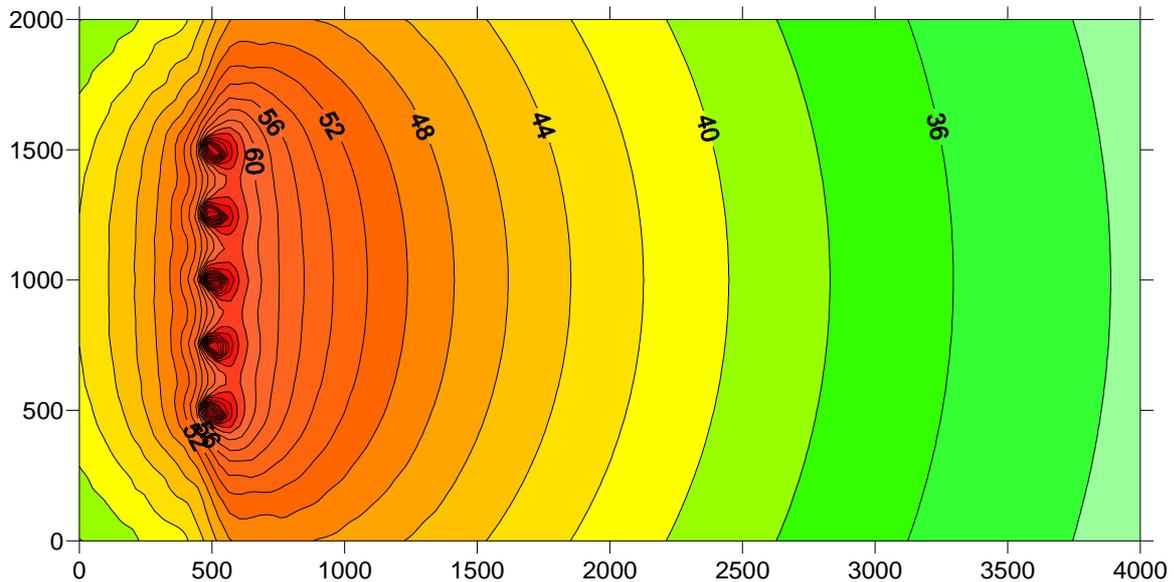
**Figure 6-3: 5 WTGs operating, all hard ground scenario**
