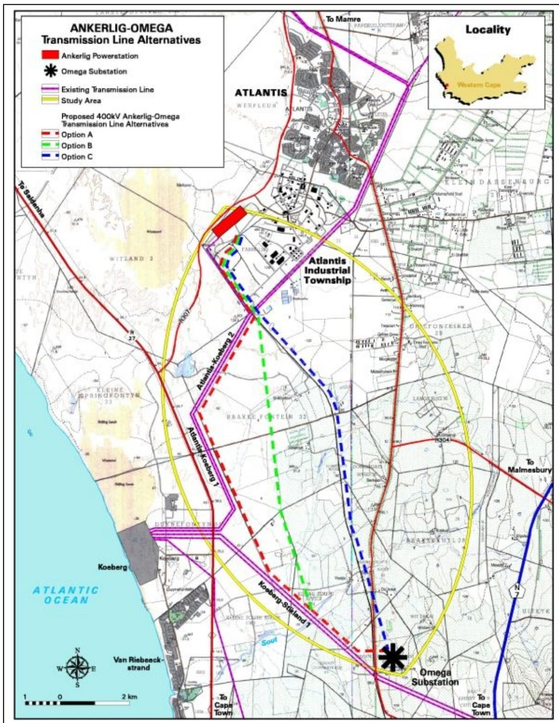
Figure 1. The three alternative routes for the Ankerlig to Omega transmission line
