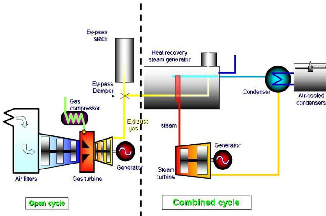
**Figure 1.1:** Simplified schematic illustrating the CCGT conversion process and components
