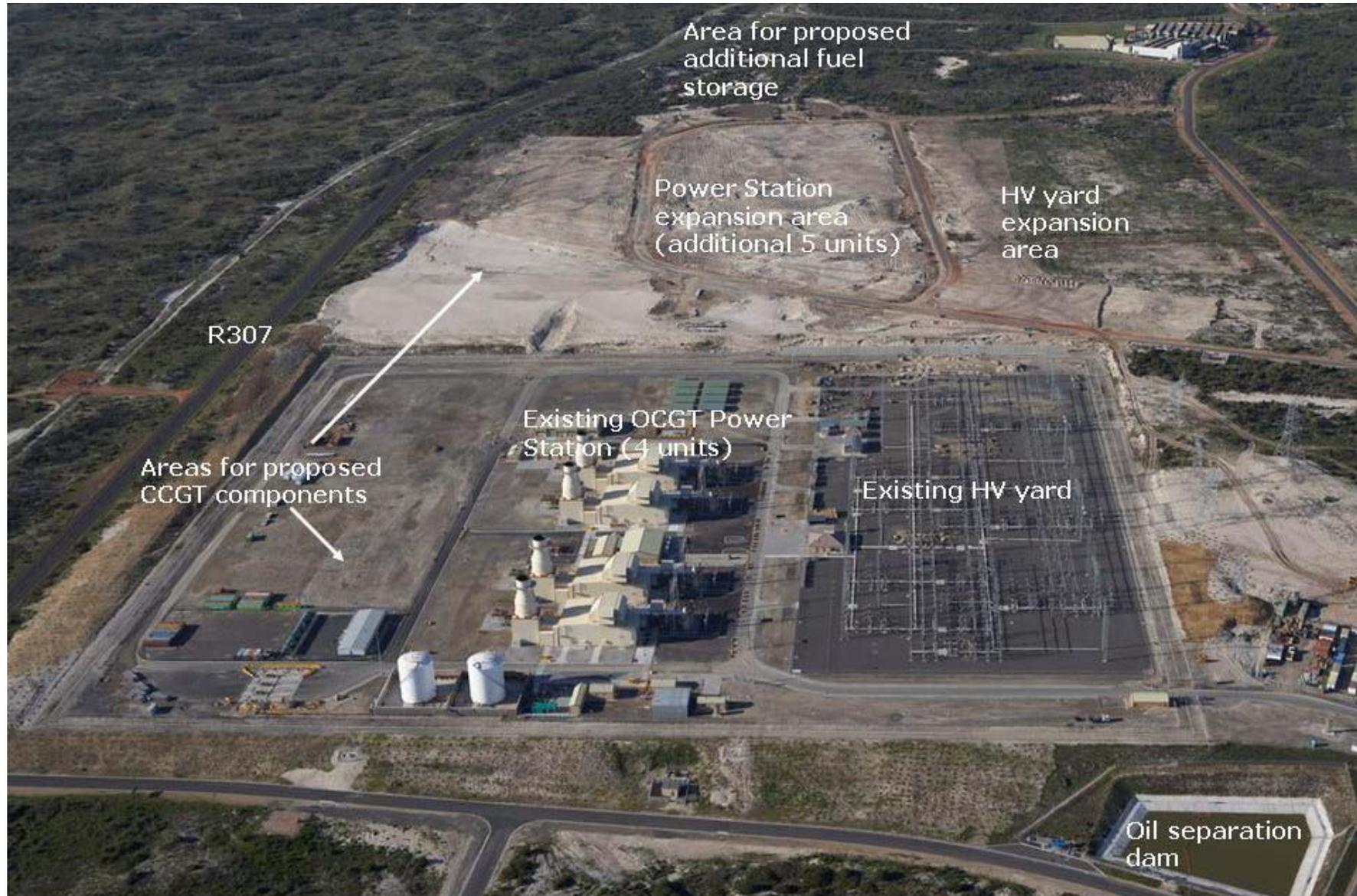
**Figure 1.2:** Aerial photograph of the Ankerlig Power Station site showing the existing power station infrastructure the power station expansion site, as well as the areas for the placement of infrastructure associated with the proposed power station conversion
