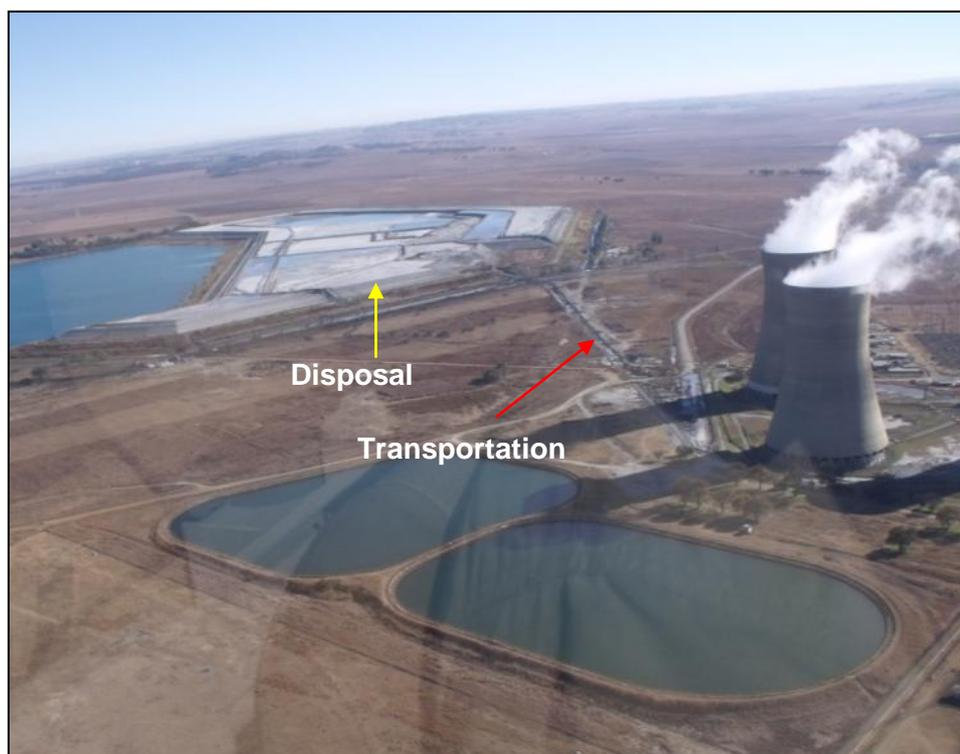
**Figure 7-6: Transportation (red) and disposal (yellow) at current ash disposal facilities.**
