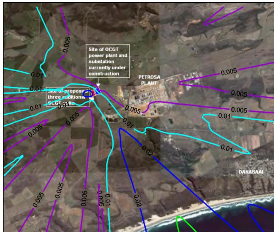
Figure A-26: Annual average predicted NO<sub>2</sub> ground level concentrations (µg/m<sup>3</sup>) for the power station (NO<sub>x</sub> 165 µg/m<sup>3</sup>, 6 units, operating 2 hours per day).
