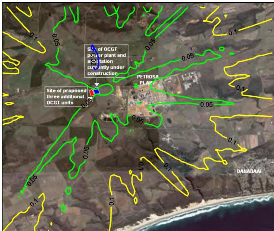
Figure A-67: Highest daily predicted SO<sub>2</sub> ground level concentrations (µg/m<sup>3</sup>) for all sources (PetroSA refinery and 6 units at power station operating 6 hours per day).
