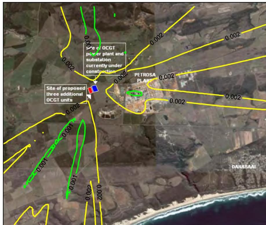
Figure A-68: Annual average predicted SO<sub>2</sub> ground level concentrations (µg/m<sup>3</sup>) for all sources (PetroSA refinery and 6 units at power station operating 6 hours per day).
