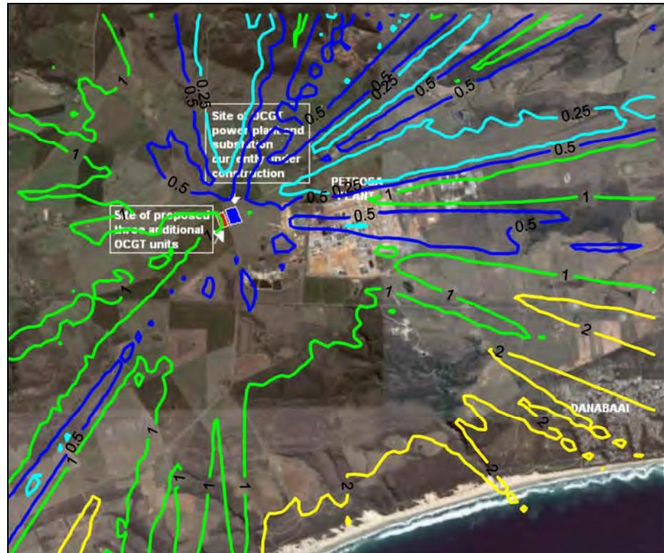
Figure A-12: Highest hourly predicted SO<sub>2</sub> ground level concentrations (µg/m<sup>3</sup>) for the power station (6 units, operating 2 hours per day).
