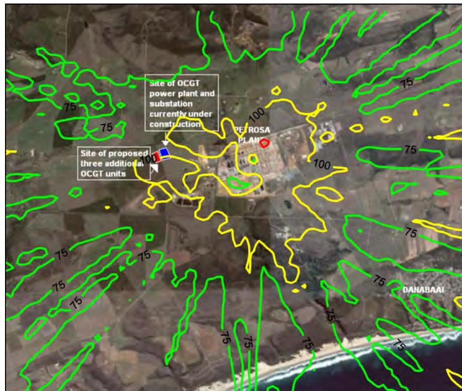
Figure A-42: Highest hourly predicted NO<sub>2</sub> ground level concentrations (µg/m<sup>3</sup>) for all sources (PetroSA refinery and 6 units at power station operating 2 hours per day).
