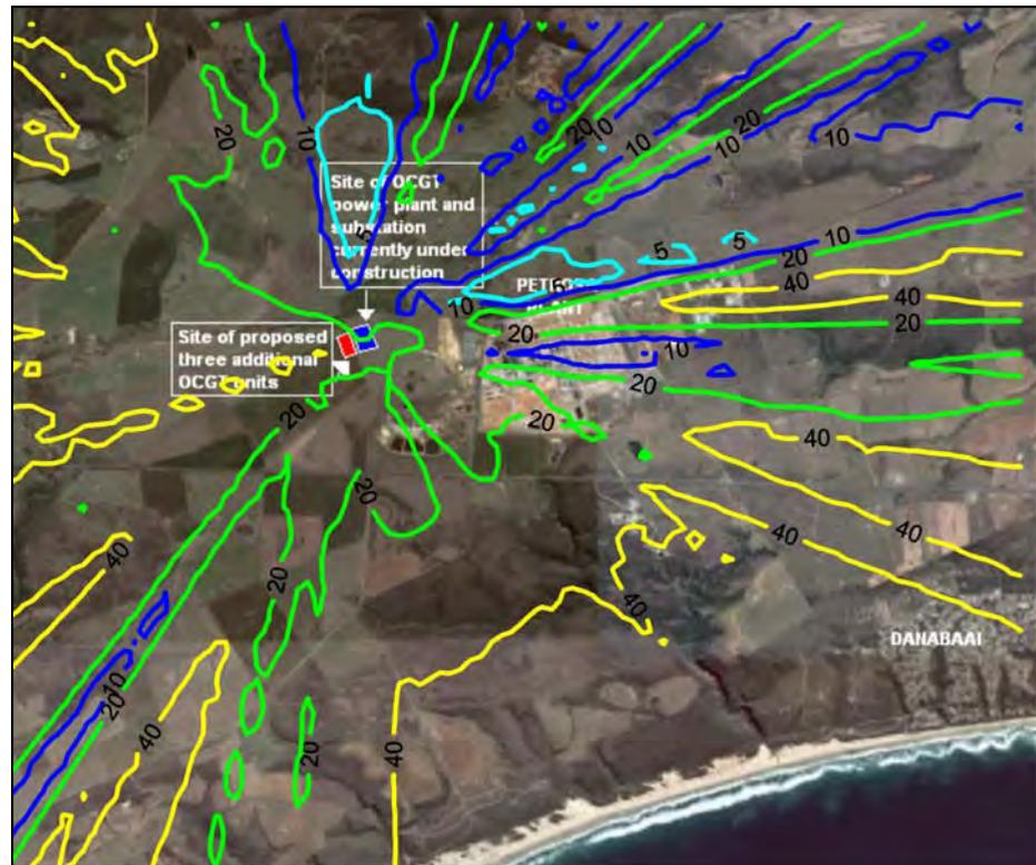
Figure A-36: Highest hourly predicted NO<sub>2</sub> ground level concentrations (µg/m<sup>3</sup>) for the power station (NO<sub>x</sub> 600 µg/m<sup>3</sup>, 6 units, operating 2 hours per day).
