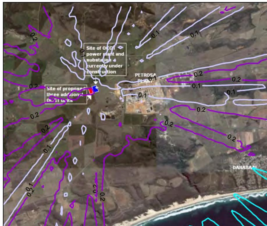
Figure A-22: Highest daily predicted NO<sub>2</sub> ground level concentrations (µg/m<sup>3</sup>) for the power station (NO<sub>x</sub> 165 µg/m<sup>3</sup>, 3 units, operating 2 hours per day).
