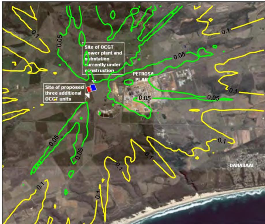
Figure A-49: Highest daily predicted PM10 ground level concentrations ( $\mu\text{g}/\text{m}^3$ ) for the power station (3 units, operating 6 hours per day).
