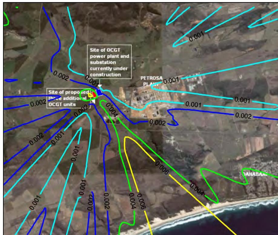
Figure A-4: Annual average predicted PM10 ground level concentrations ( $\mu\text{g}/\text{m}^3$ ) for the power station (6 units, operating 2 hours per day).
