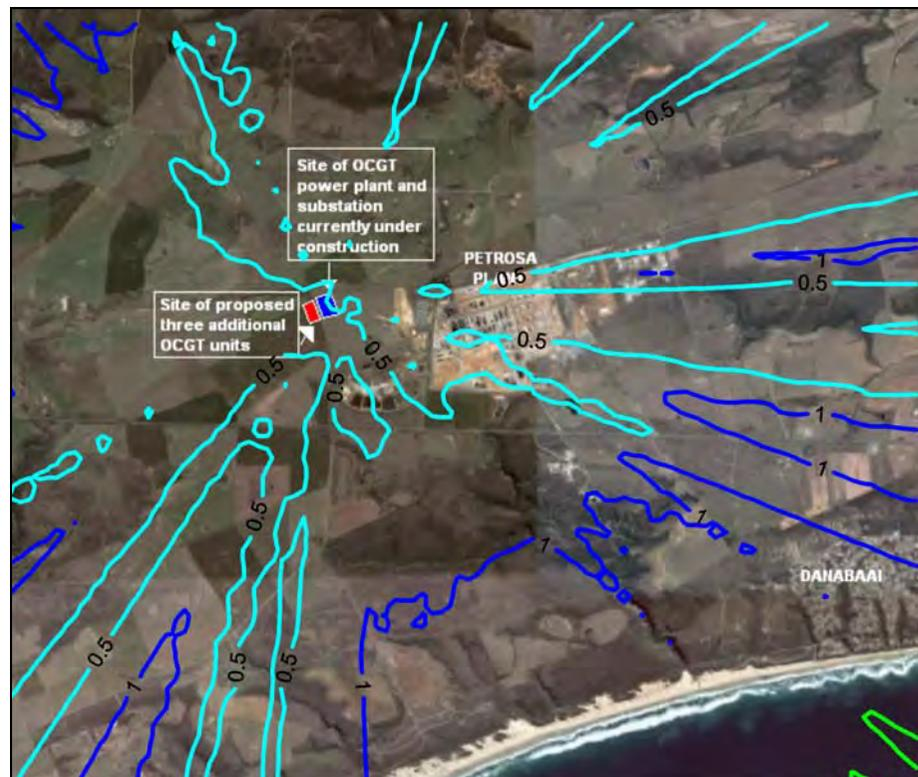
Figure A-34: Highest daily predicted NO<sub>2</sub> ground level concentrations (µg/m<sup>3</sup>) for the power station (NO<sub>x</sub> 600 µg/m<sup>3</sup>, 3 units, operating 2 hours per day).
