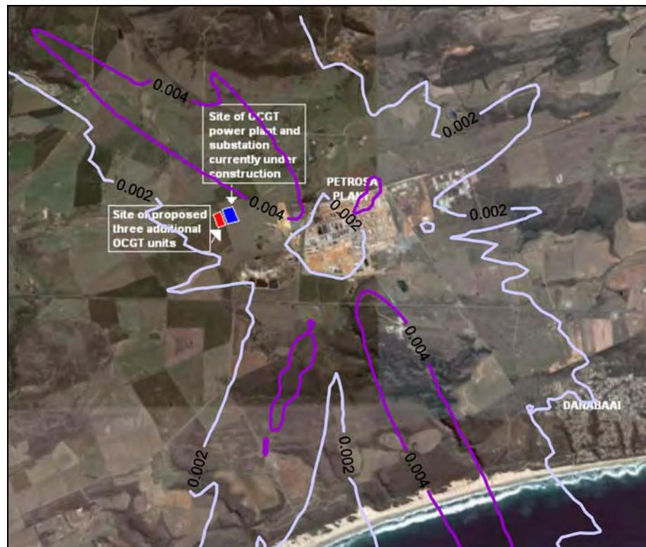
Figure A-16: Highest daily predicted SO<sub>2</sub> ground level concentrations (µg/m<sup>3</sup>) for the PetroSA refinery.
