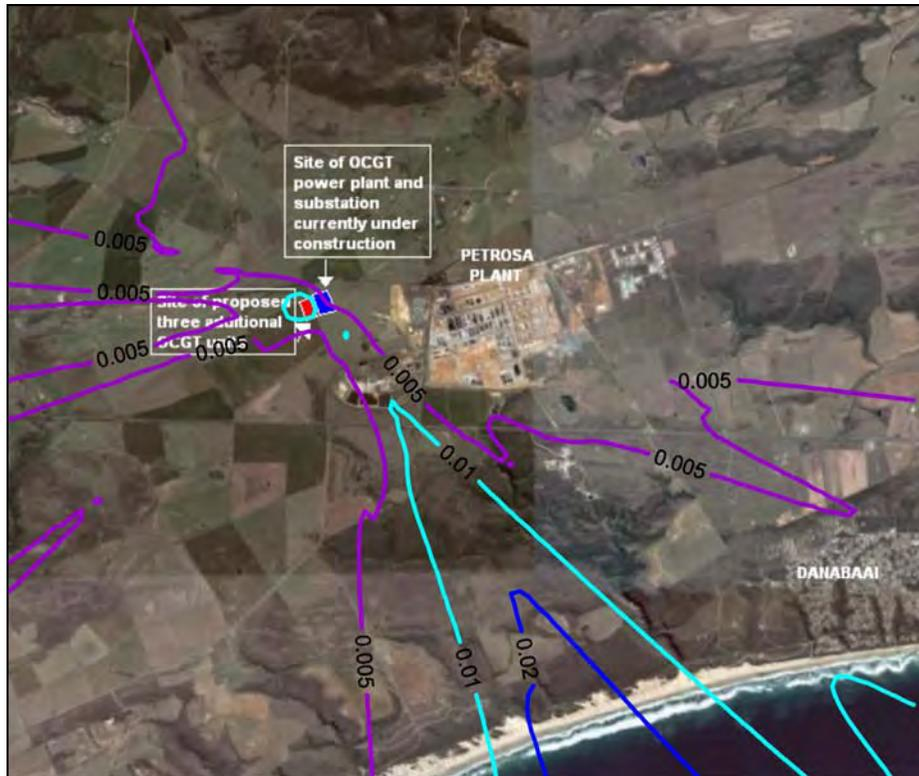
Figure A-23: Annual average predicted NO<sub>2</sub> ground level concentrations (µg/m<sup>3</sup>) for the power station (NO<sub>x</sub> 165 µg/m<sup>3</sup>, 3 units, operating 2 hours per day).
