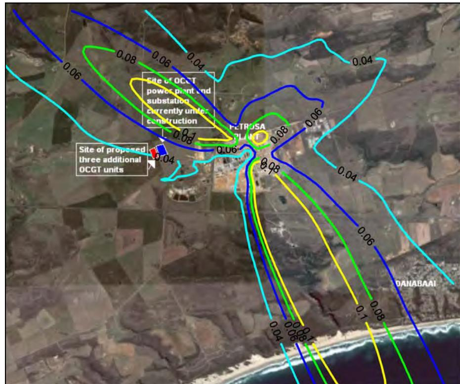
Figure A-6: Annual average predicted PM10 ground level concentrations ( $\mu\text{g}/\text{m}^3$ ) for the PetroSA refinery.
