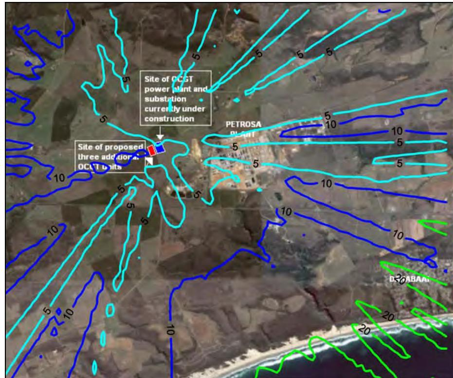
Figure A-24: Highest hourly predicted NO<sub>2</sub> ground level concentrations (µg/m<sup>3</sup>) for the power station (NO<sub>x</sub> 165 µg/m<sup>3</sup>, 6 units, operating 2 hours per day).
