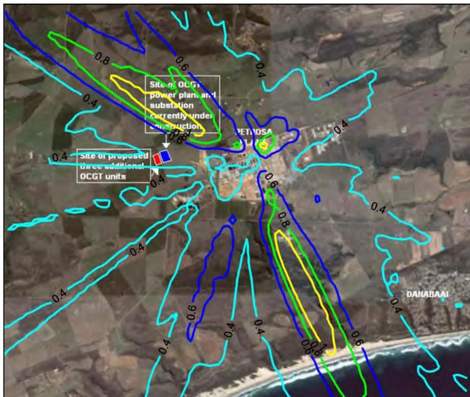
Figure A-7: Highest daily predicted PM10 ground level concentrations ( $\mu\text{g}/\text{m}^3$ ) for all sources (PetroSA refinery and 6 units at power station operating 2 hours per day).
