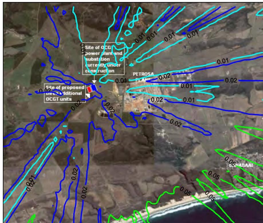
Figure A-10: Highest daily predicted SO<sub>2</sub> ground level concentrations (µg/m<sup>3</sup>) for the power station (3 units, operating 2 hours per day).
