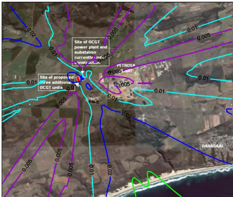
Figure A-71: Annual average predicted NO<sub>2</sub> ground level concentrations ( $\mu\text{g}/\text{m}^3$ ) for the power station (NO<sub>x</sub> 165  $\mu\text{g}/\text{m}^3$ , 3 units, operating 6 hours per day).
