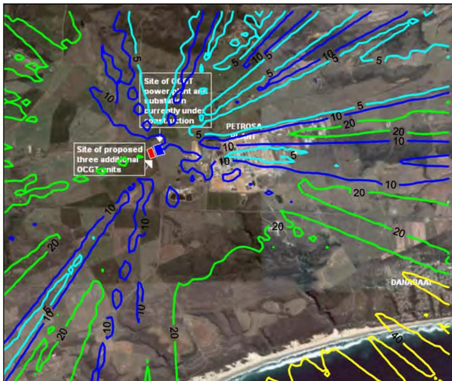
Figure A-33: Highest hourly predicted NO<sub>2</sub> ground level concentrations (µg/m<sup>3</sup>) for the power station (NO<sub>x</sub> 600 µg/m<sup>3</sup>, 3 units, operating 2 hours per day).
