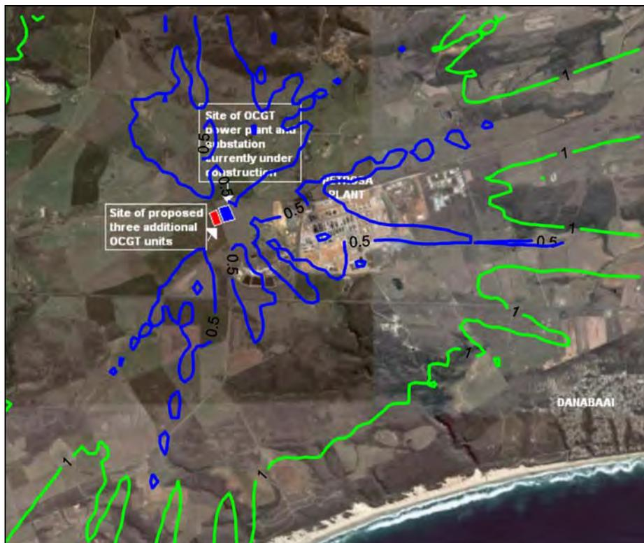
Figure A-57: Highest hourly predicted SO<sub>2</sub> ground level concentrations (µg/m<sup>3</sup>) for the power station (3 units, operating 6 hours per day).
