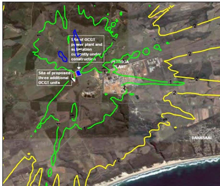
Figure A-60: Highest hourly predicted SO<sub>2</sub> ground level concentrations (µg/m<sup>3</sup>) for the power station (6 units, operating 6 hours per day).
