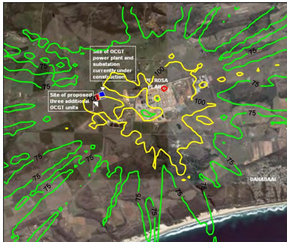
Figure A-30: Highest hourly predicted NO<sub>2</sub> ground level concentrations (µg/m<sup>3</sup>) for all sources (PetroSA refinery and 6 units at power station operating 2 hours per day).
