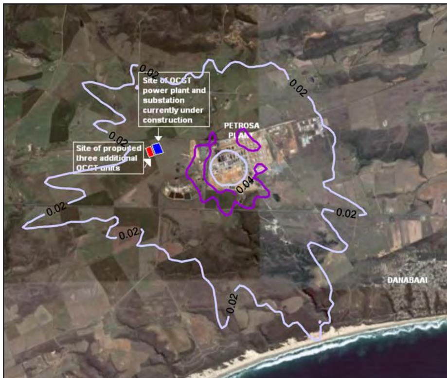
Figure A-15: Highest hourly predicted SO<sub>2</sub> ground level concentrations (µg/m<sup>3</sup>) for the PetroSA refinery.
