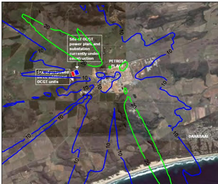
Figure A-43: Highest daily predicted NO<sub>2</sub> ground level concentrations (µg/m<sup>3</sup>) for all sources (PetroSA refinery and 6 units at power station operating 2 hours per day).
