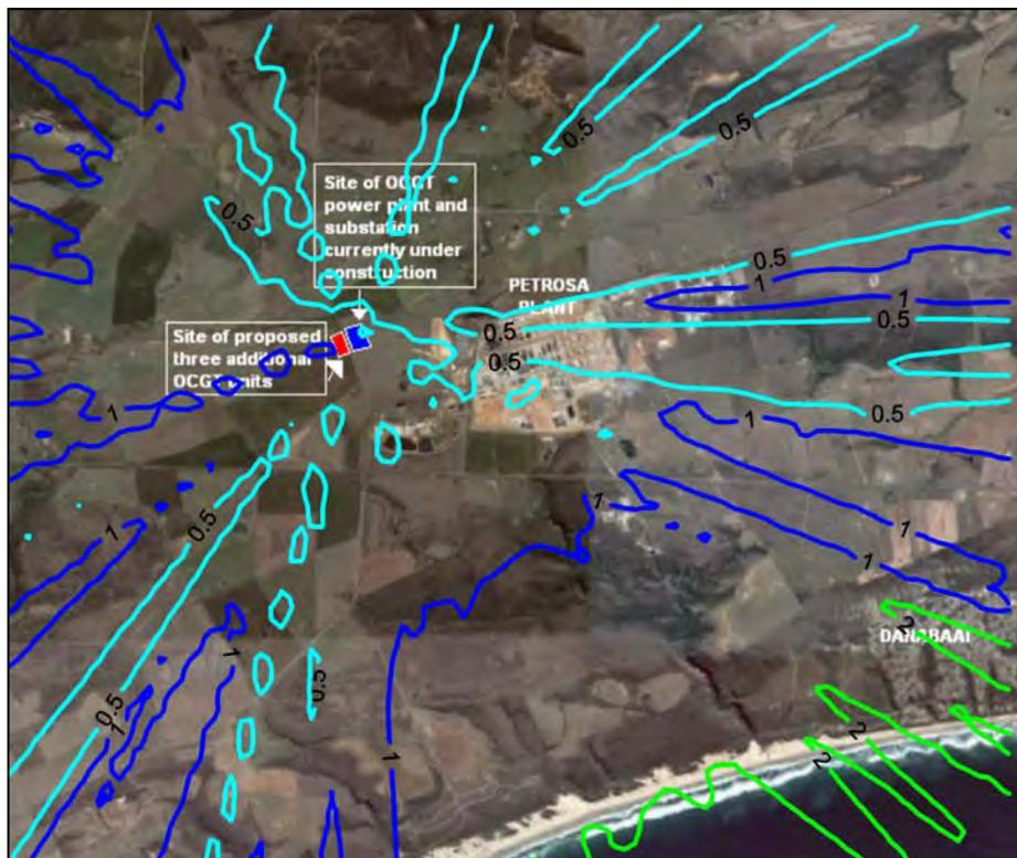
Figure A-45: Highest hourly predicted CO ground level concentrations ( $\mu\text{g}/\text{m}^3$ ) for the power station (3 units, operating 2 hours per day).
