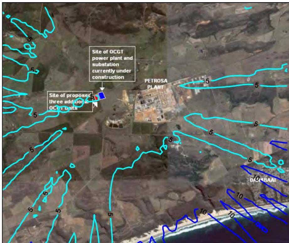
Figure A-21: Highest hourly predicted NO<sub>2</sub> ground level concentrations (µg/m<sup>3</sup>) for the power station (NO<sub>x</sub> 165 µg/m<sup>3</sup>, 3 units, operating 2 hours per day).
