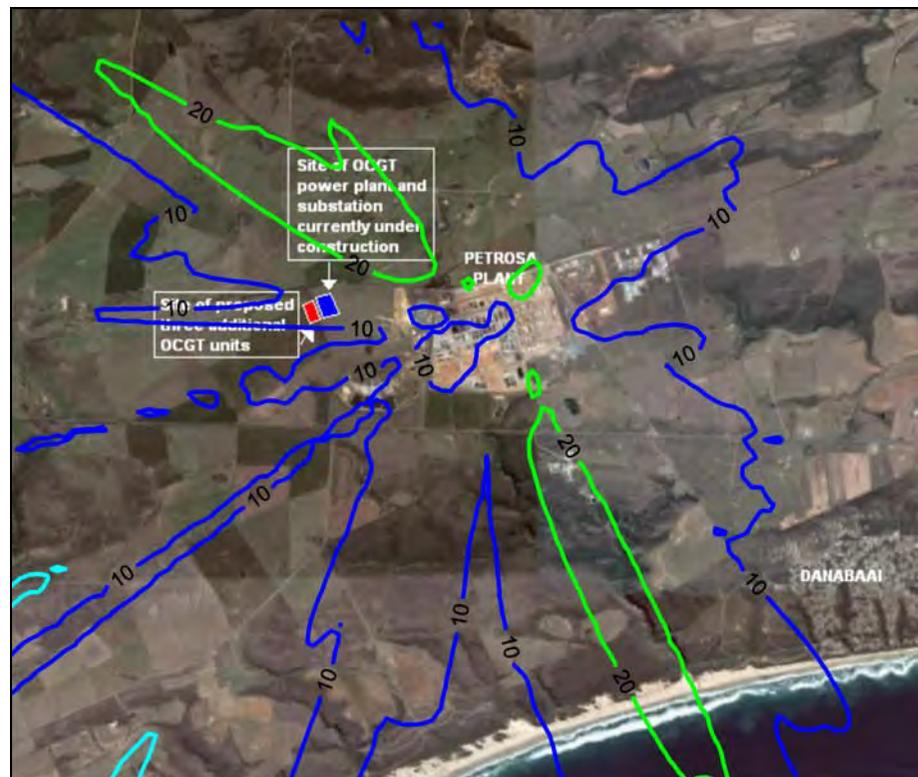
Figure A-40: Highest daily predicted NO<sub>2</sub> ground level concentrations (µg/m<sup>3</sup>) for the PetroSA refinery.
