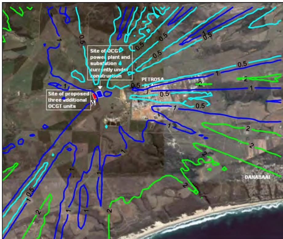
Figure A-37: Highest daily predicted NO<sub>2</sub> ground level concentrations (µg/m<sup>3</sup>) for the power station (NO<sub>x</sub> 600 µg/m<sup>3</sup>, 6 units, operating 2 hours per day).
