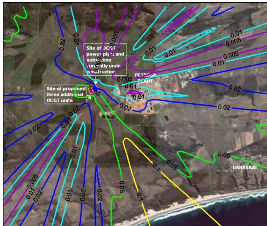
Figure A-38: Annual average predicted NO<sub>2</sub> ground level concentrations (µg/m<sup>3</sup>) for the power station (NO<sub>x</sub> 600 µg/m<sup>3</sup>, 6 units, operating 2 hours per day).
