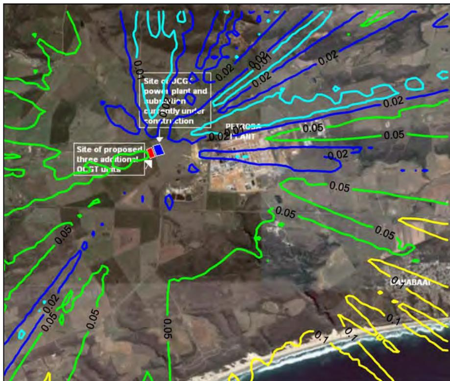
Figure A-19: Highest daily predicted SO<sub>2</sub> ground level concentrations (µg/m<sup>3</sup>) for all sources (PetroSA refinery and 6 units at power station operating 2 hours per day).
