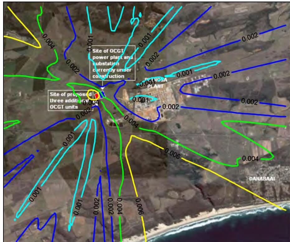
Figure A-50: Annual average predicted PM10 ground level concentrations ( $\mu\text{g}/\text{m}^3$ ) for the power station (3 units, operating 6 hours per day).
