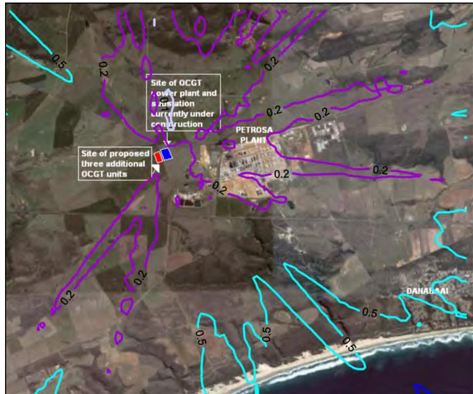
Figure A-70: Highest daily predicted NO<sub>2</sub> ground level concentrations (µg/m<sup>3</sup>) for the power station (NO<sub>x</sub> 165 µg/m<sup>3</sup>, 3 units, operating 6 hours per day).
