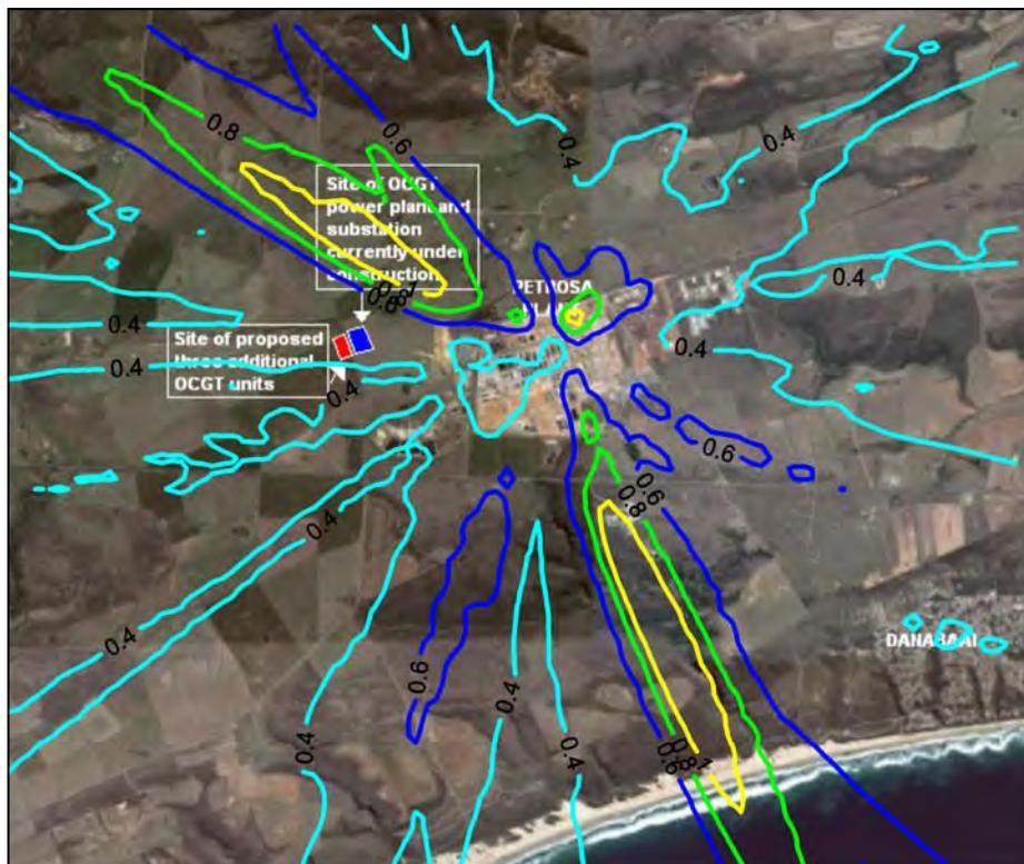
Figure A-55: Highest daily predicted PM10 ground level concentrations ( $\mu\text{g}/\text{m}^3$ ) for all sources (PetroSA refinery and 6 units at power station operating 6 hours per day).
