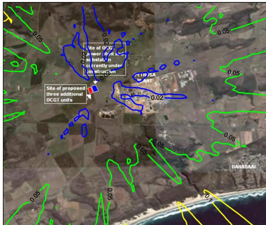
Figure A-58: Highest daily predicted SO<sub>2</sub> ground level concentrations (µg/m<sup>3</sup>) for the power station (3 units, operating 6 hours per day).
