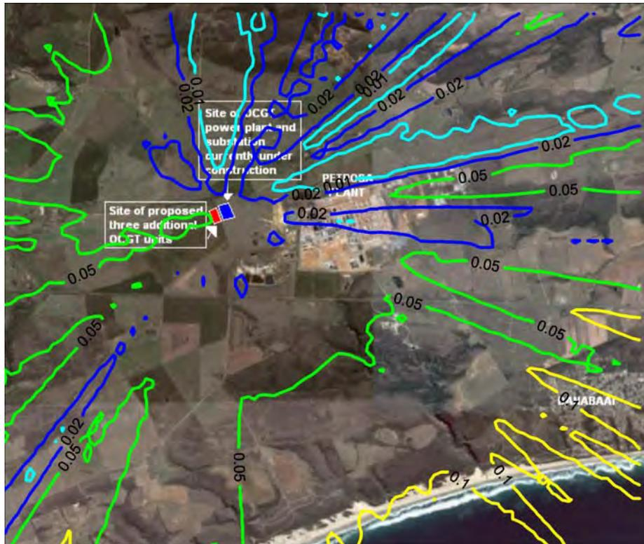
Figure A-13: Highest daily predicted SO<sub>2</sub> ground level concentrations (µg/m<sup>3</sup>) for the power station (6 units, operating 2 hours per day).
