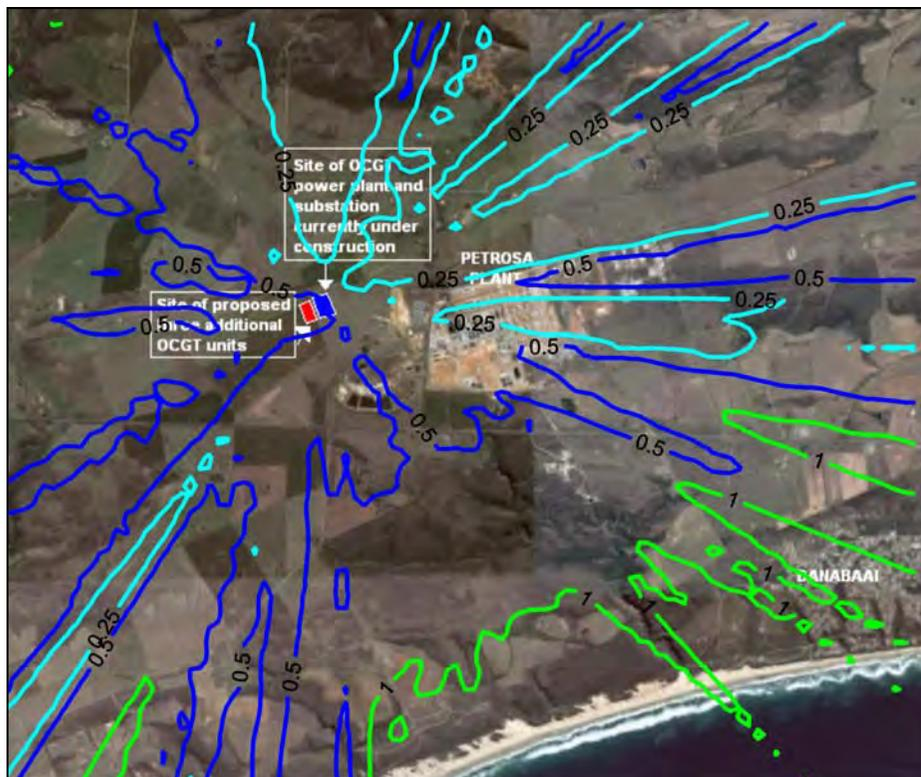
Figure A-9: Highest hourly predicted SO<sub>2</sub> ground level concentrations (µg/m<sup>3</sup>) for the power station (3 units, operating 2 hours per day).
