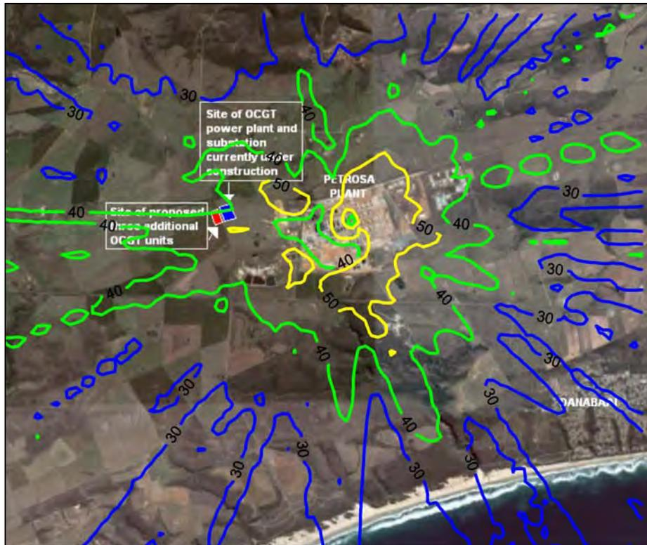
Figure A-47: Highest hourly predicted CO ground level concentrations ( $\mu\text{g}/\text{m}^3$ ) for the PetroSA refinery.
