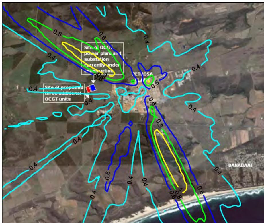
Figure A-53: Highest daily predicted PM10 ground level concentrations ( $\mu\text{g}/\text{m}^3$ ) for the PetroSA refinery.
