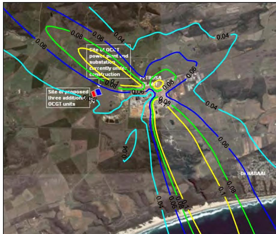
Figure A-8: Annual average predicted PM10 ground level concentrations ( $\mu\text{g}/\text{m}^3$ ) for all sources (PetroSA refinery and 6 units at power station operating 2 hours per day).
