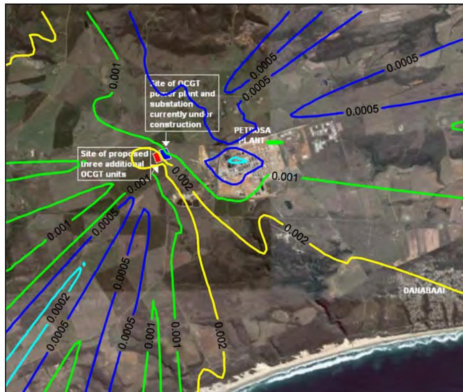
Figure A-20: Annual average predicted SO<sub>2</sub> ground level concentrations (µg/m<sup>3</sup>) for all sources (PetroSA refinery and 6 units at power station operating 2 hours per day).
