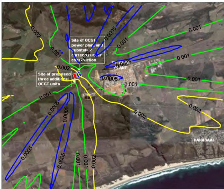
Figure A-59: Annual average predicted SO<sub>2</sub> ground level concentrations (µg/m<sup>3</sup>) for the power station (3 units, operating 6 hours per day).
