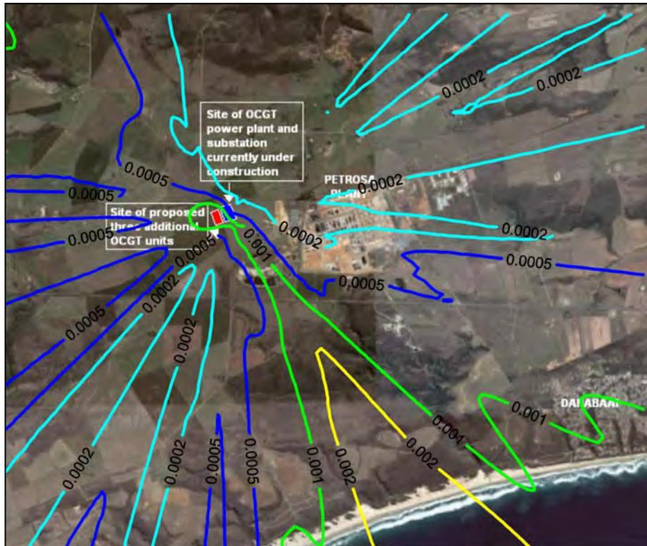
Figure A-11: Annual average predicted SO<sub>2</sub> ground level concentrations (µg/m<sup>3</sup>) for the power station (3 units, operating 2 hours per day).
