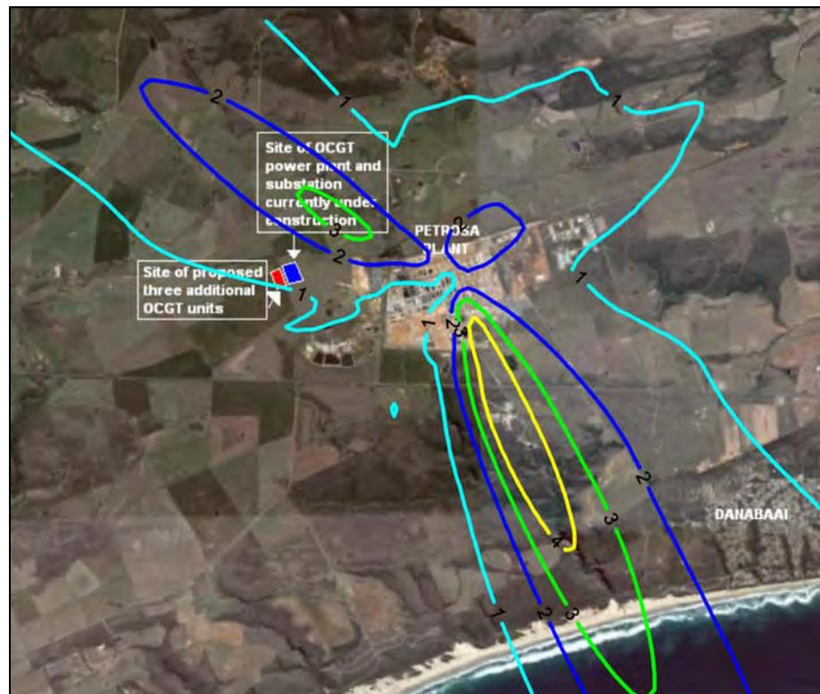
Figure A-32: Annual average predicted NO<sub>2</sub> ground level concentrations (µg/m<sup>3</sup>) for all sources (PetroSA refinery and 6 units at power station operating 2 hours per day).
