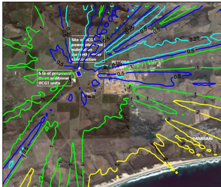
Figure A-18: Highest hourly predicted SO<sub>2</sub> ground level concentrations (µg/m<sup>3</sup>) for all sources (PetroSA refinery and 6 units at power station operating 2 hours per day).
