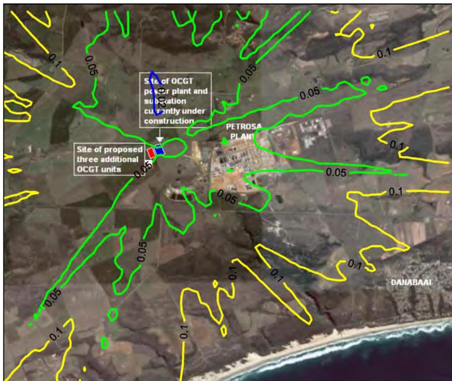
Figure A-61: Highest daily predicted SO<sub>2</sub> ground level concentrations (µg/m<sup>3</sup>) for the power station (6 units, operating 6 hours per day).
