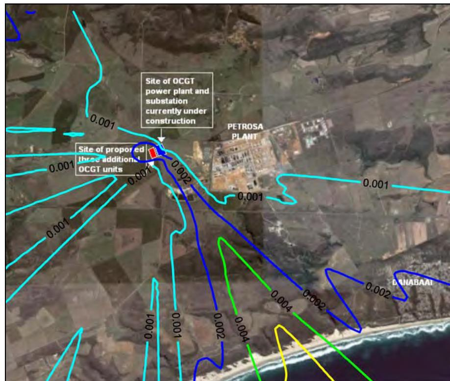
Figure A-2: Annual average predicted PM10 ground level concentrations ( $\mu\text{g}/\text{m}^3$ ) for the power station (3 units, operating 2 hours per day).
