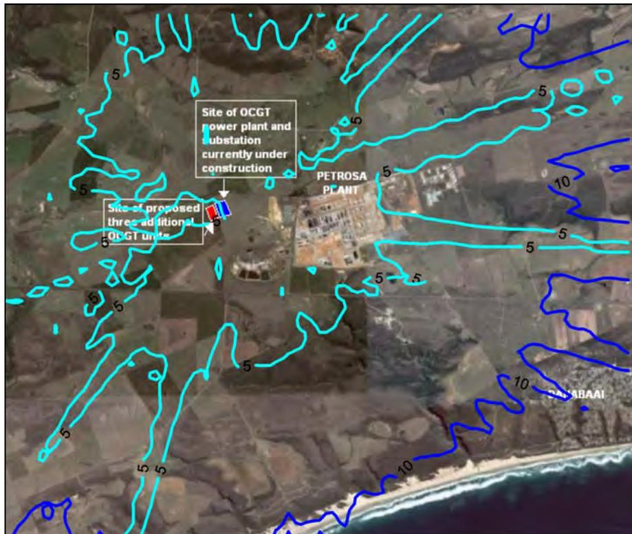
Figure A-69: Highest hourly predicted NO<sub>2</sub> ground level concentrations (µg/m<sup>3</sup>) for the power station (NO<sub>x</sub> 165 µg/m<sup>3</sup>, 3 units, operating 6 hours per day).
