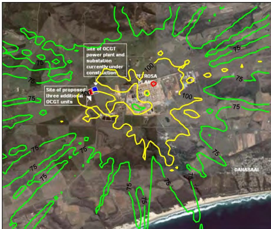
Figure A-27: Highest hourly predicted NO<sub>2</sub> ground level concentrations (µg/m<sup>3</sup>) for the PetroSA refinery.
