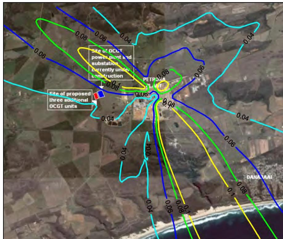
Figure A-56: Annual average predicted PM10 ground level concentrations ( $\mu\text{g}/\text{m}^3$ ) for all sources (PetroSA refinery and 6 units at power station operating 6 hours per day).
