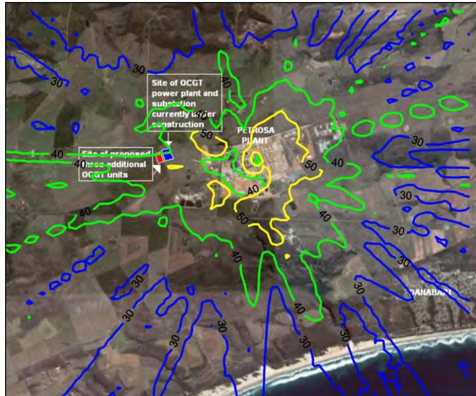
Figure A-48: Highest hourly predicted CO ground level concentrations ( $\mu\text{g}/\text{m}^3$ ) for all sources (PetroSA refinery and 6 units at power station operating 2 hours per day).
