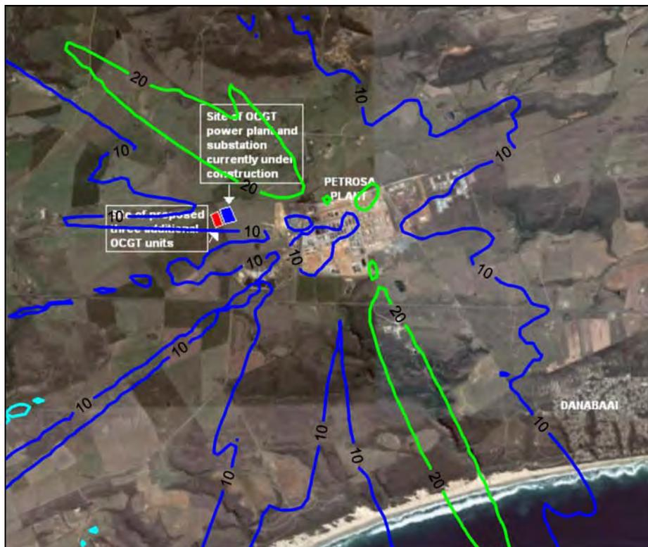
Figure A-31: Highest daily predicted NO<sub>2</sub> ground level concentrations (µg/m<sup>3</sup>) for all sources (PetroSA refinery and 6 units at power station operating 2 hours per day).
