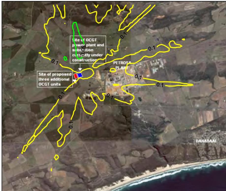
Figure A-51: Highest daily predicted PM10 ground level concentrations ( $\mu\text{g}/\text{m}^3$ ) for the power station (6 units, operating 6 hours per day).
