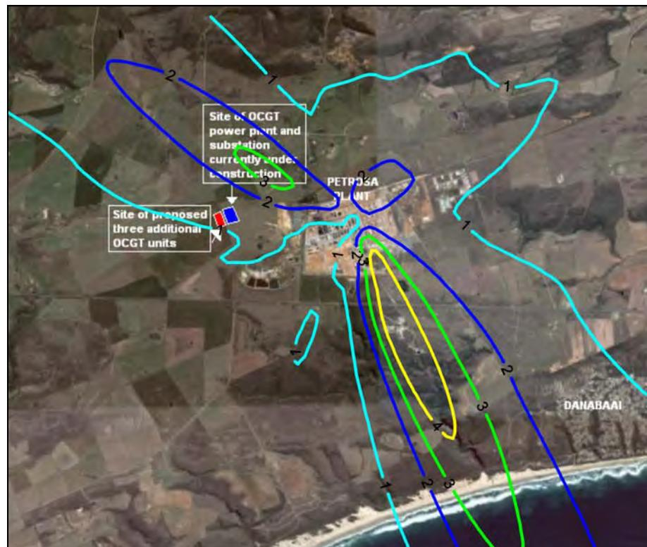
Figure A-44: Annual average predicted NO<sub>2</sub> ground level concentrations (µg/m<sup>3</sup>) for all sources (PetroSA refinery and 6 units at power station operating 2 hours per day).
