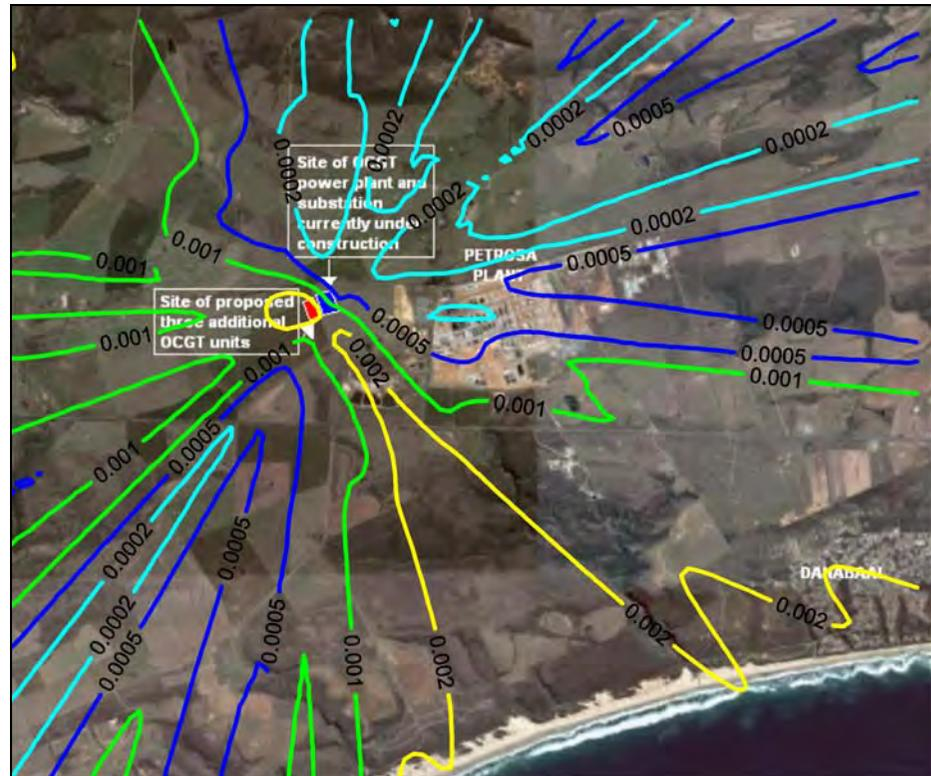
Figure A-14: Annual average predicted SO<sub>2</sub> ground level concentrations (µg/m<sup>3</sup>) for the power station (6 units, operating 2 hours per day).
