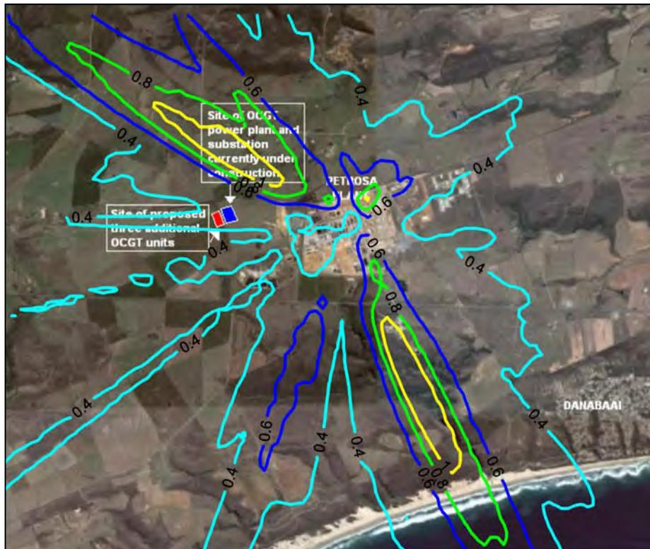
Figure A-5: Highest daily predicted PM10 ground level concentrations ( $\mu\text{g}/\text{m}^3$ ) for the PetroSA refinery.
