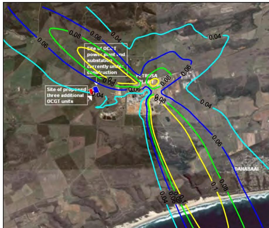
Figure A-54: Annual average predicted PM10 ground level concentrations ( $\mu\text{g}/\text{m}^3$ ) for the PetroSA refinery.
