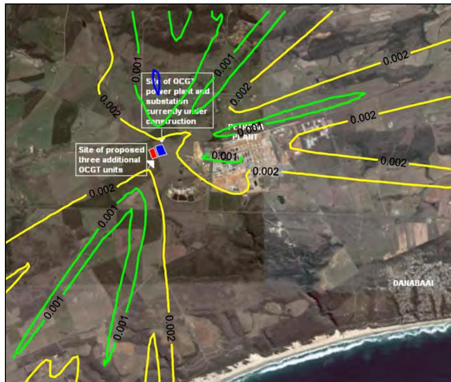
Figure A-62: Annual average predicted SO<sub>2</sub> ground level concentrations (µg/m<sup>3</sup>) for the power station (6 units, operating 6 hours per day).
