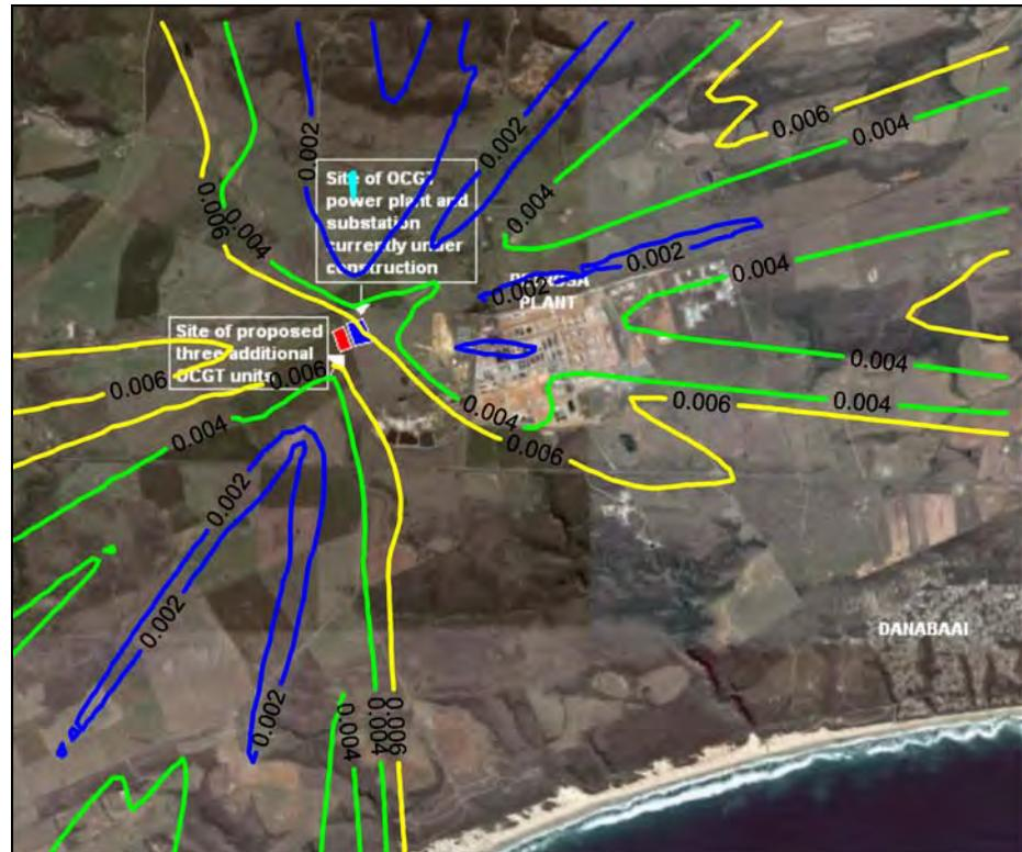
Figure A-52: Annual average predicted PM10 ground level concentrations ( $\mu\text{g}/\text{m}^3$ ) for the power station (6 units, operating 6 hours per day).
