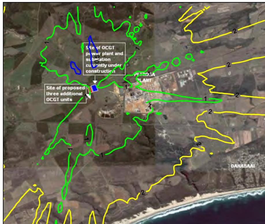
Figure A-66: Highest hourly predicted SO<sub>2</sub> ground level concentrations (µg/m<sup>3</sup>) for all sources (PetroSA refinery and 6 units at power station operating 6 hours per day).
