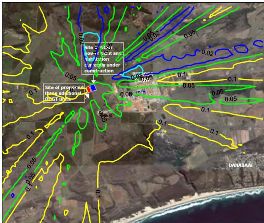
Figure A-3: Highest daily predicted PM10 ground level concentrations ( $\mu\text{g}/\text{m}^3$ ) for the power station (6 units, operating 2 hours per day).
