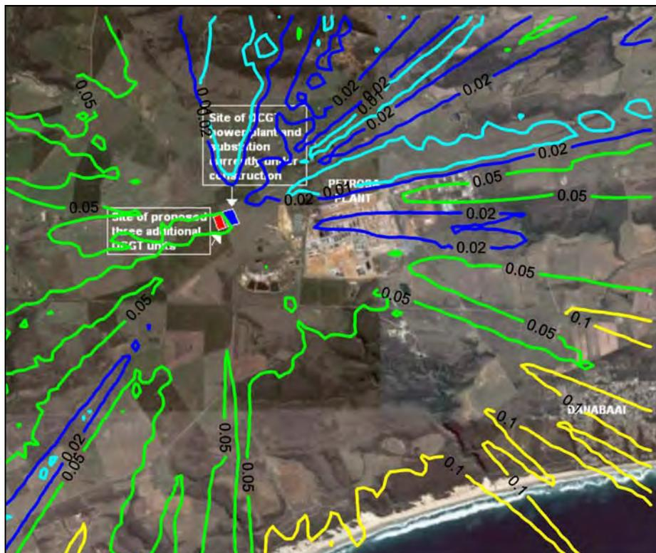
Figure A-1: Highest daily predicted PM10 ground level concentrations ( $\mu\text{g}/\text{m}^3$ ) for the power station (3 units, operating 2 hours per day).
