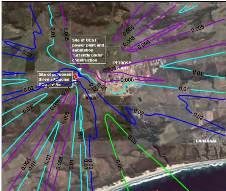
Figure A-35: Annual average predicted NO<sub>2</sub> ground level concentrations (µg/m<sup>3</sup>) for the power station (NO<sub>x</sub> 600 µg/m<sup>3</sup>, 3 units, operating 2 hours per day).
