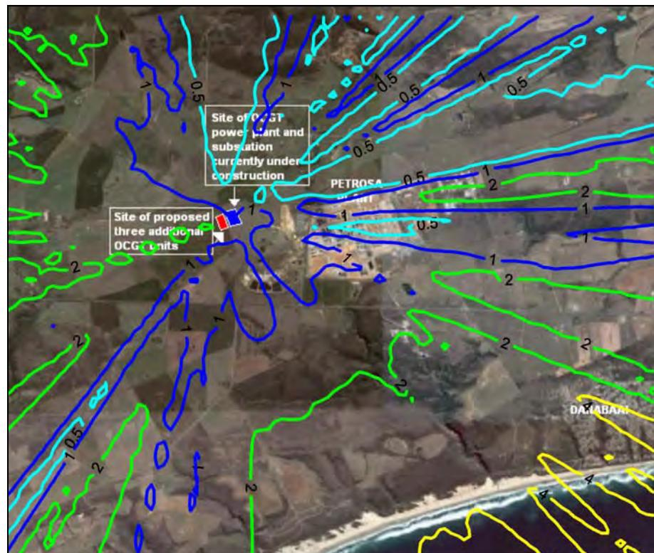
Figure A-46: Highest hourly predicted CO ground level concentrations ( $\mu\text{g}/\text{m}^3$ ) for the power station (6 units, operating 2 hours per day).
