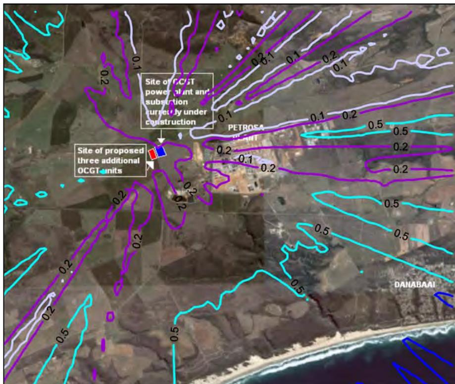
Figure A-25: Highest daily predicted NO<sub>2</sub> ground level concentrations (µg/m<sup>3</sup>) for the power station (NO<sub>x</sub> 165 µg/m<sup>3</sup>, 6 units, operating 2 hours per day).
