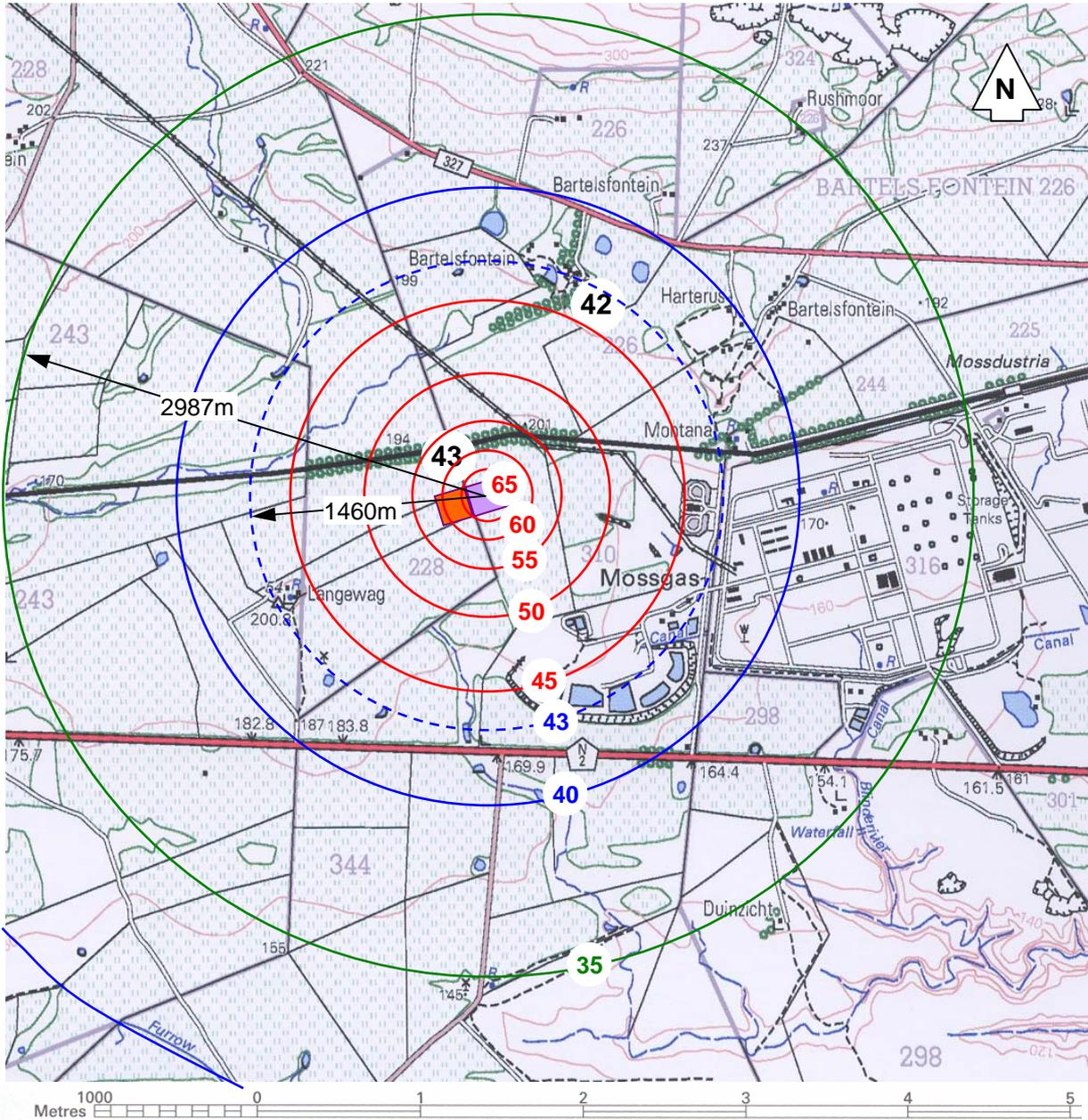
**FIGURE 6**  $L_{Req,d}$  for three existing OCGT units operating 5 hours during daytime
