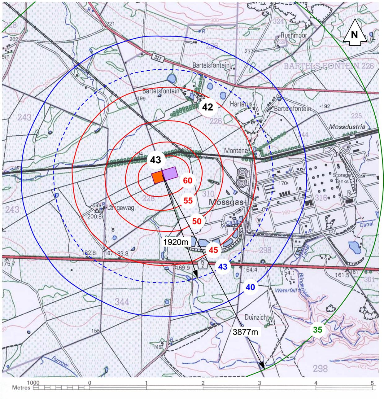
**FIGURE 8**  $L_{Req,d}$  for six OCGT units operating 5 hours during daytime
