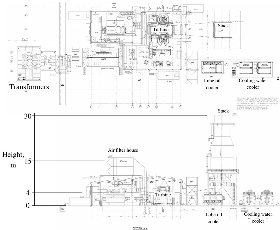
**FIGURE 4** Plan and section of an OCGT power generation unit
