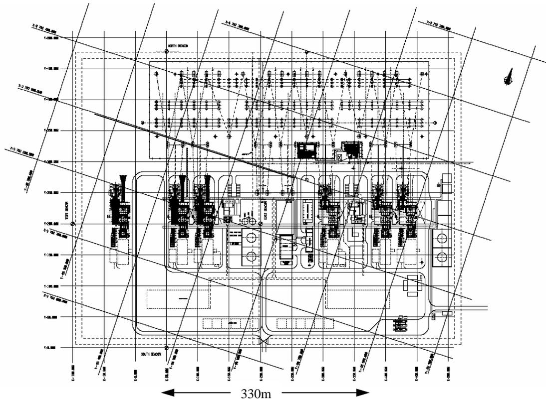
**FIGURE 2** Site plan showing three OCGT under construction to the right and the proposed three additional OCGT units to the left
