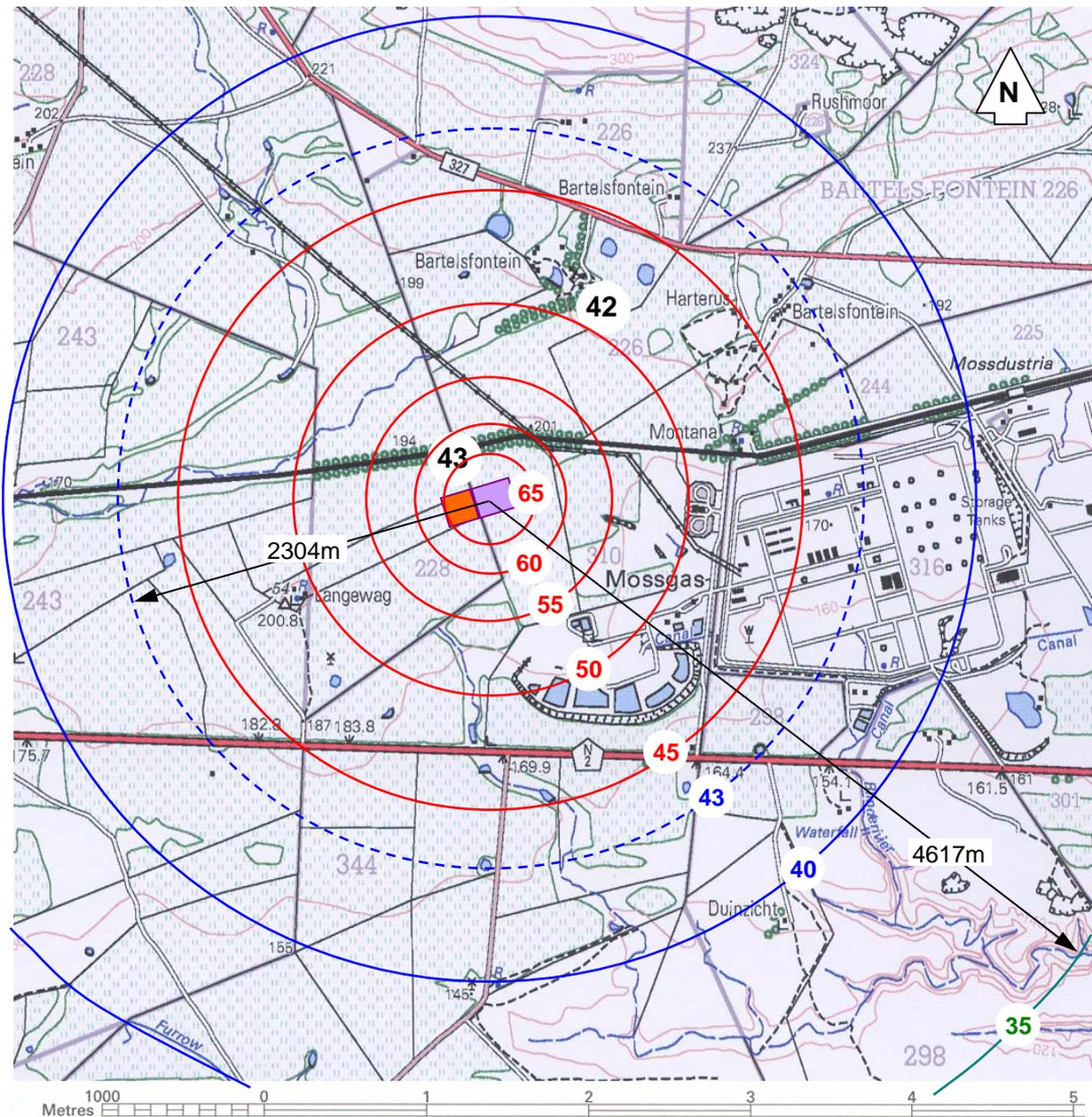
**FIGURE 5**  $L_{Req,T}$  for three existing OCGT units operating continuously
