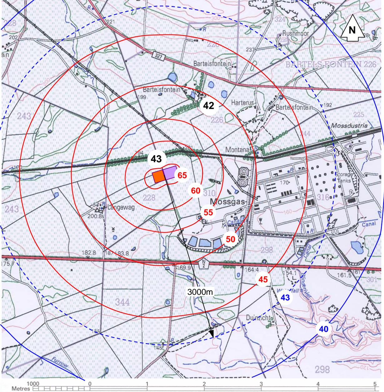
**FIGURE 7**  $L_{Req,T}$  for six OCGT units operating continuously
