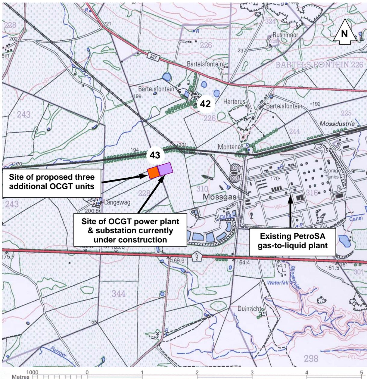
**Figure 1** Study area showing the Site of OCGT power plant & substation currently under construction and the site for the proposed three additional OCGT units
