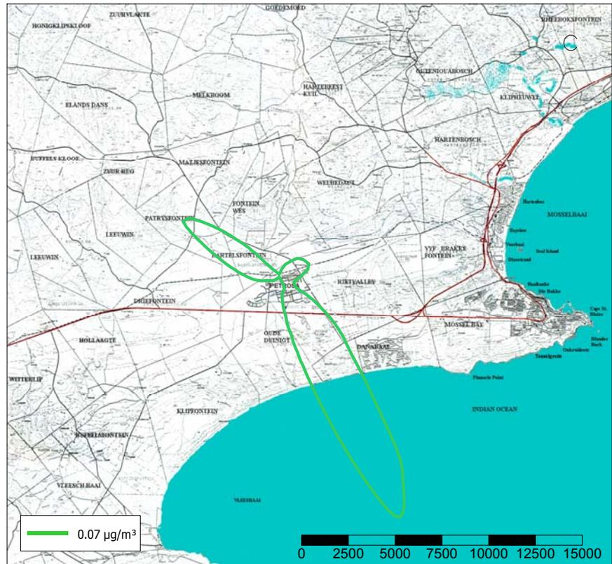
**Figure C-6 Annual average predicted PM10 ground level concentrations ( $\mu\text{g}/\text{m}^3$ ) for all sources.**
