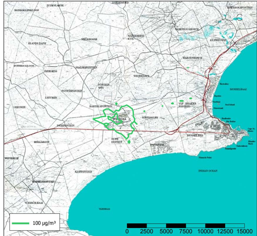
Figure C-22 Highest hourly predicted NO<sub>2</sub> ground level concentrations (µg/m<sup>3</sup>) for all sources.
