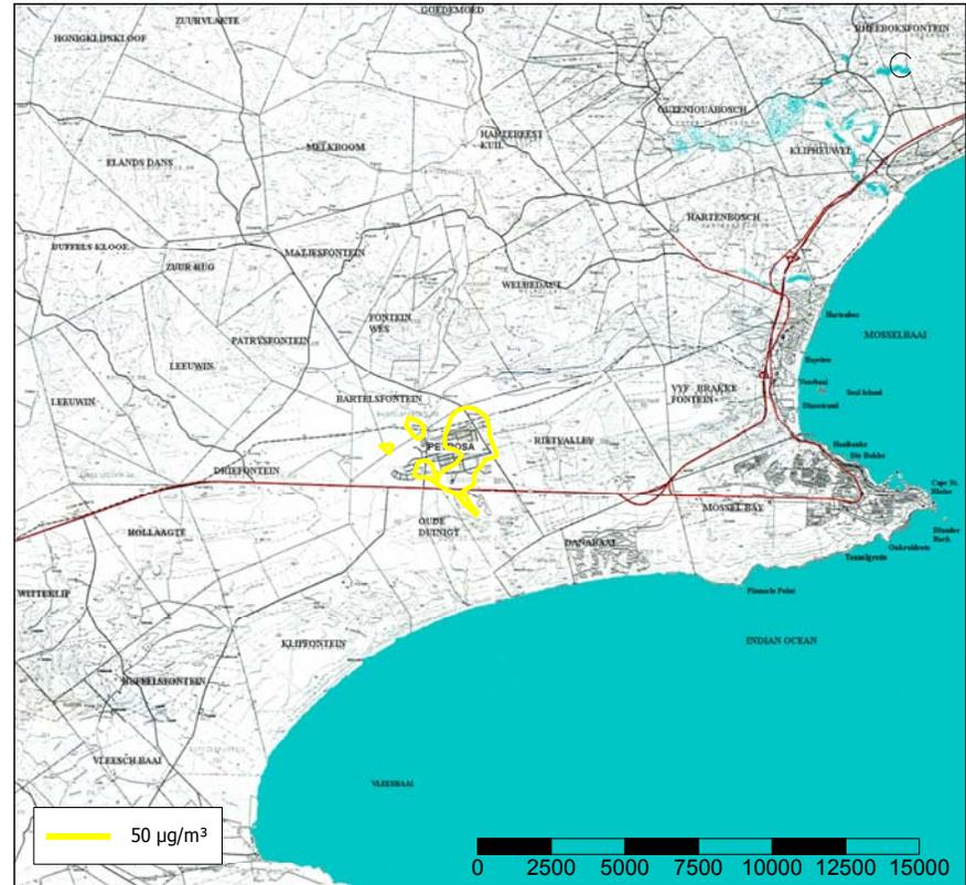
**Figure C-26 Highest hourly predicted CO ground level concentrations ( $\mu\text{g}/\text{m}^3$ ) for the PetroSA refinery (baseline).**
