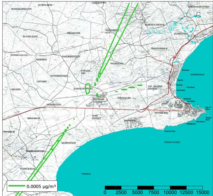
**Figure C-18 Annual average predicted NO<sub>2</sub> ground level concentrations (µg/m<sup>3</sup>) for the power station.**
