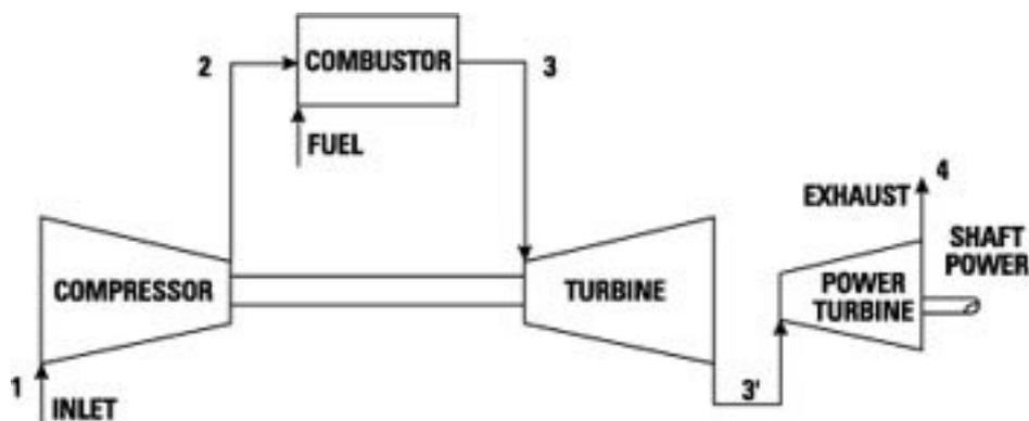
Figure 1: Schematic representation of a power generation gas turbine (Langston & Opdyke, Jr., 1997).
