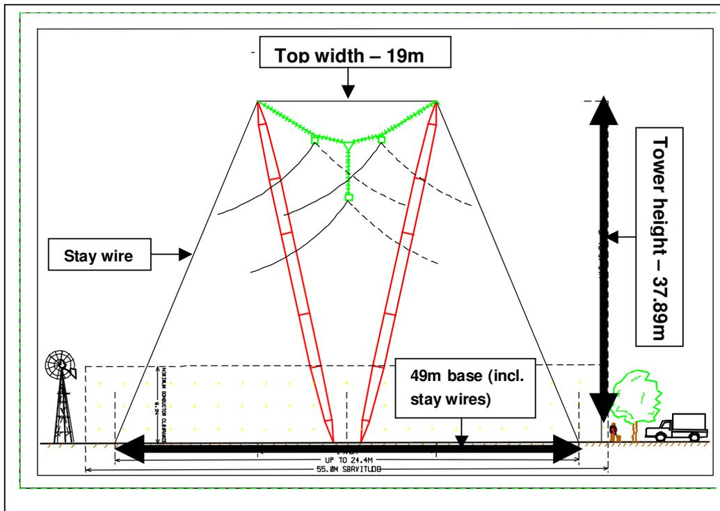
Figure 6: Diagrammatic representation of the compact cross-rope suspension tower configuration
