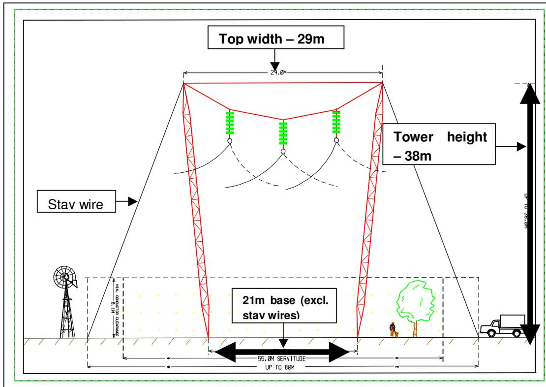
Figure 7: Diagrammatic representation of the cross-rope suspension tower Configuration
