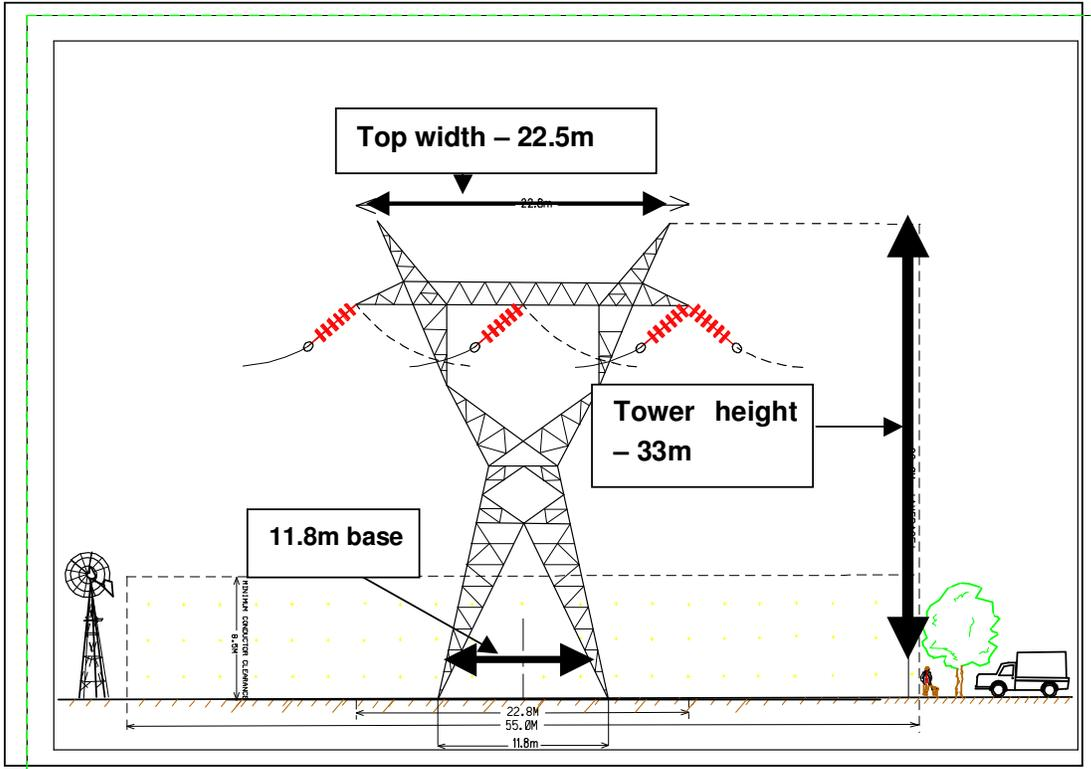
Figure 8: Diagrammatic representation of the self supporting strain tower configuration
