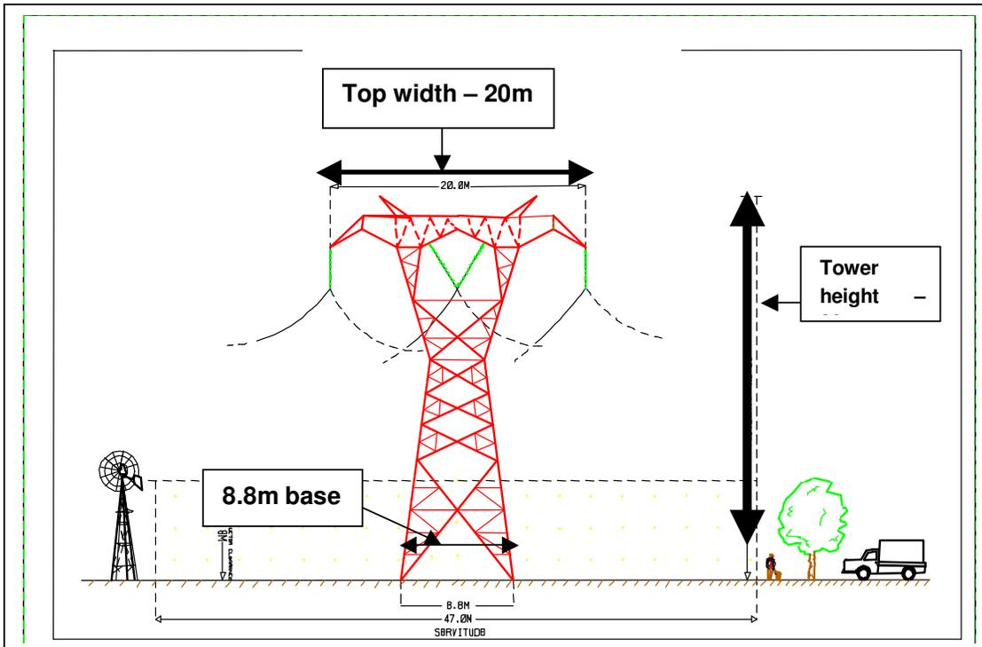
Figure 9: Diagrammatic representation of the self supporting tower configuration
