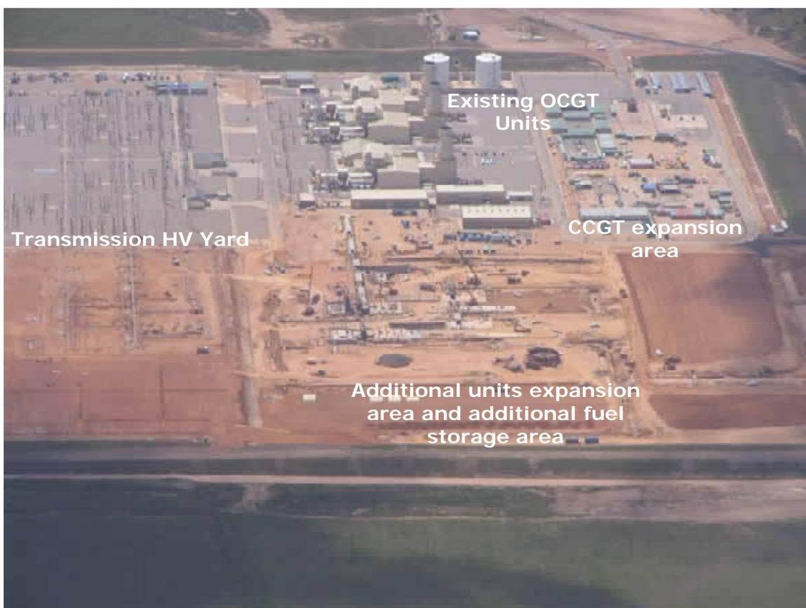
**Figure 1.3:** Aerial photograph of the Gourikwa Power Station site showing the existing power station infrastructure, the power station expansion site, as well as the areas for the placement of infrastructure associated with the proposed power station conversion
