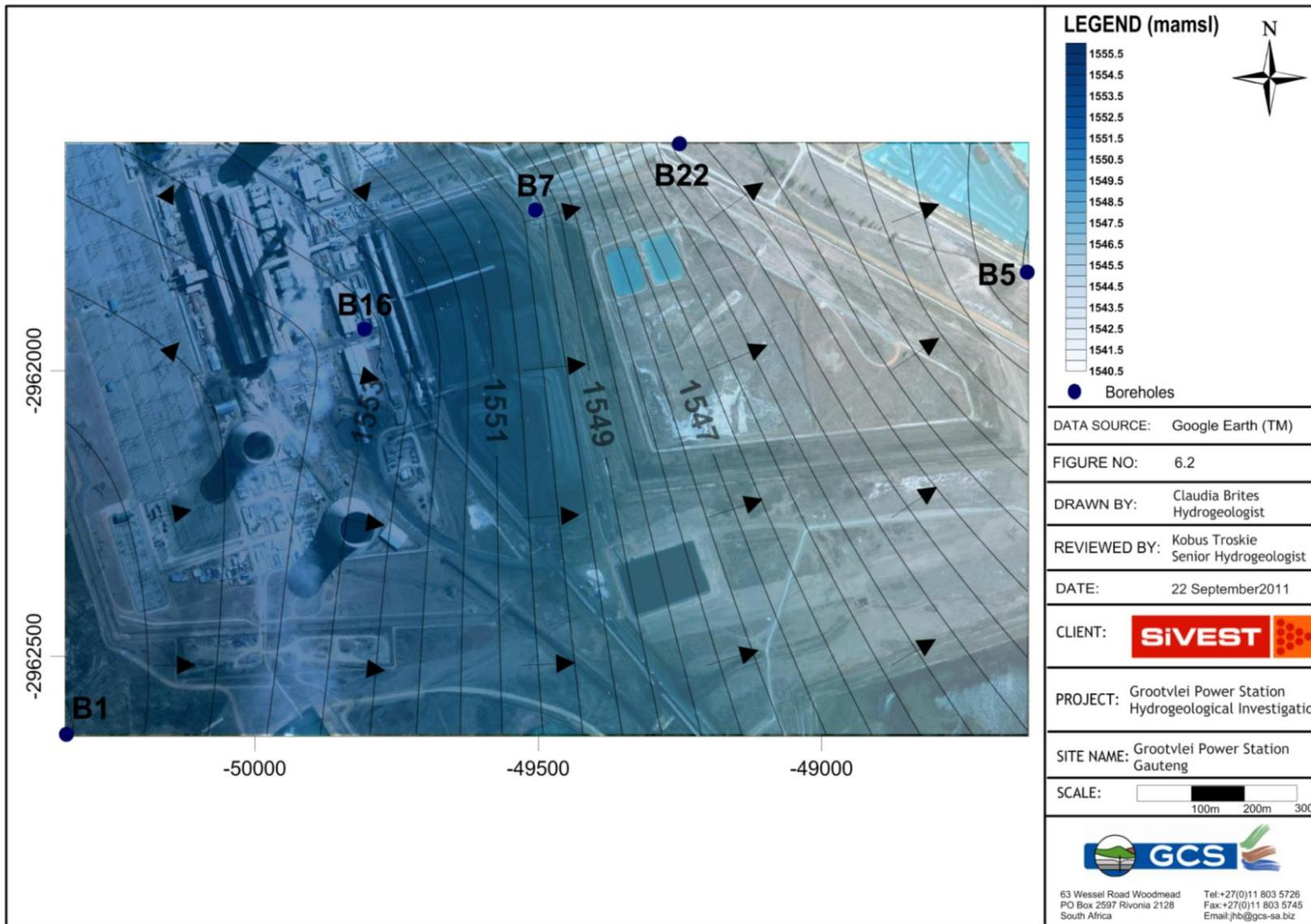
Figure 6-2: Groundwater Flow Directions
