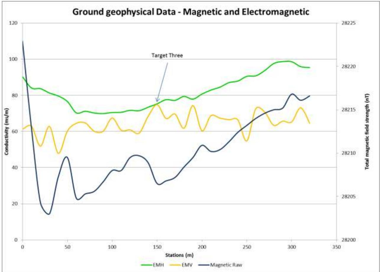
Figure 3-6 Graph indicating em and magnetic raw data surveyed on Line four
