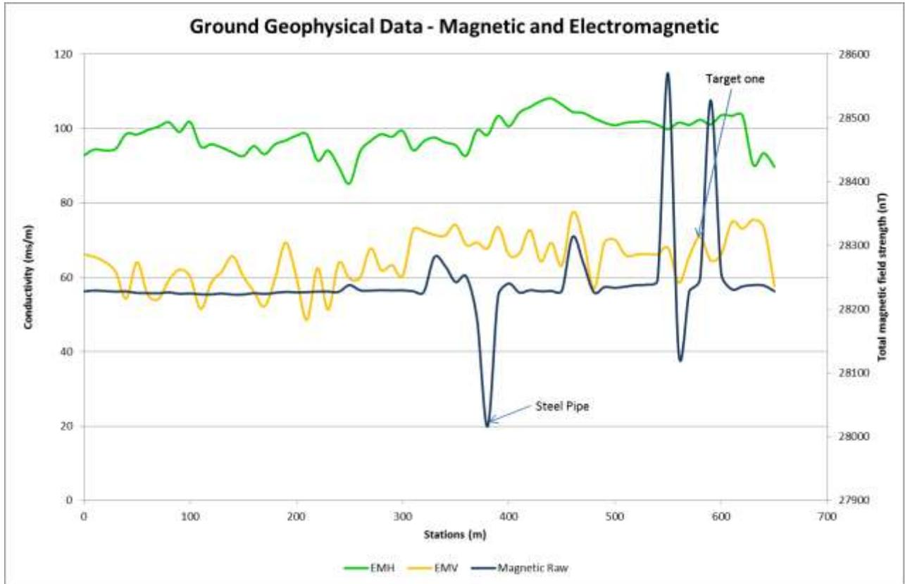
**Figure 3-3 Graph indicating em and magnetic raw data surveyed on Line one**
