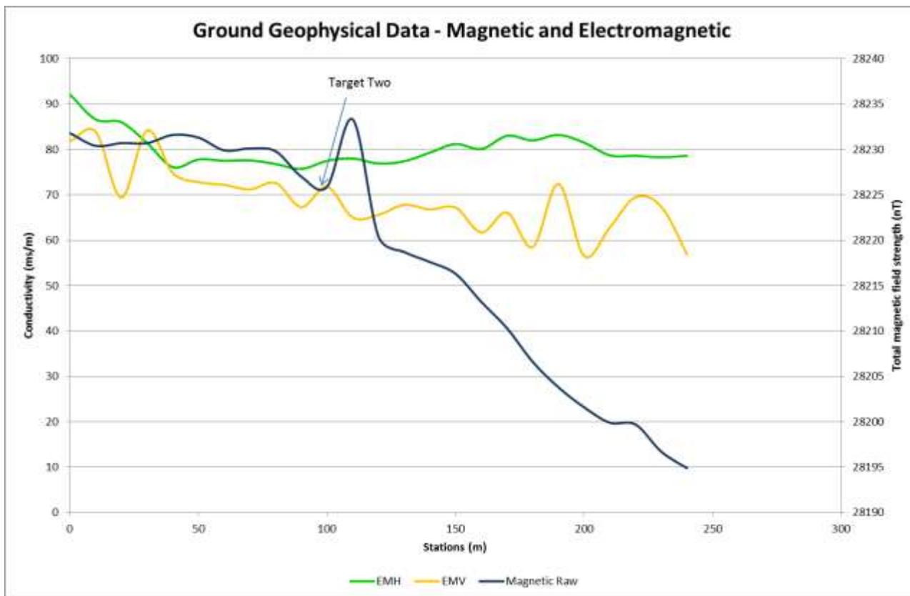
Figure 3-4 Graph indicating em and magnetic raw data surveyed on Line two
