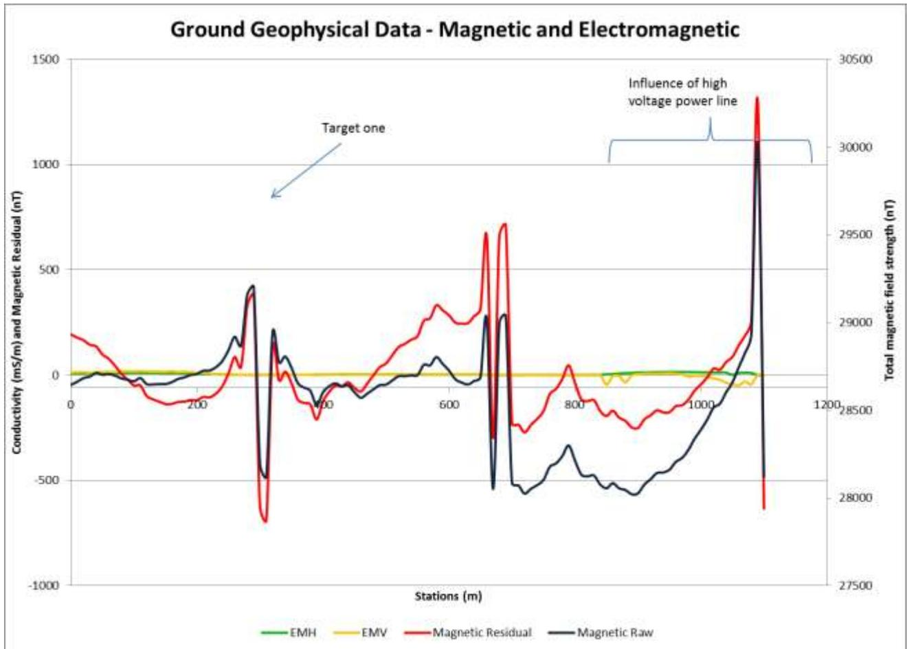
Figure 3-2 Graph indicating an example of the magnetic residual data used for interpretation
