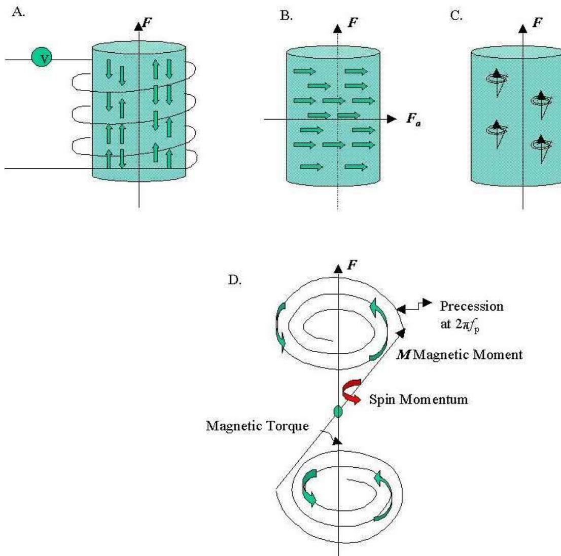
Figure 3-1 Basic operating principles of a proton magnetometer (After Kearey and Brooks, 1991)
