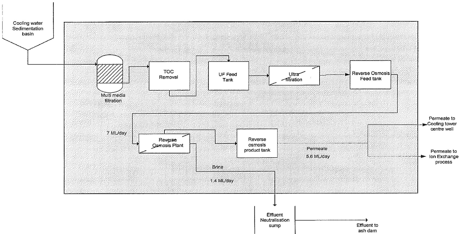
Figure 3: Flow diagram of proposed RO plant process (shaded grey) at Hendrina Power Station, Mpumalanga
