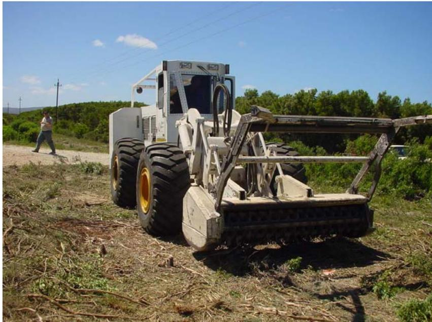
**Figure 2.** An example of a mechanical mulching machine.
