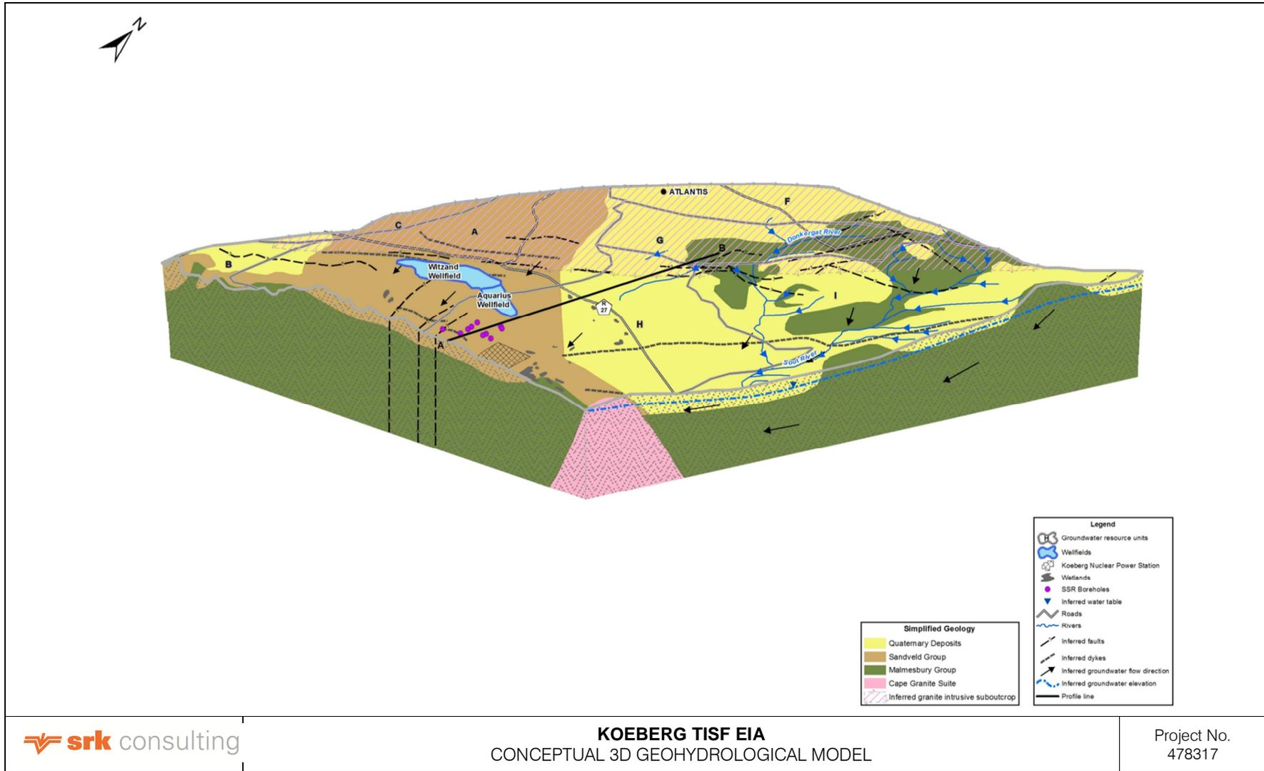
Figure 4-9: Conceptual 3D geohydrological model
