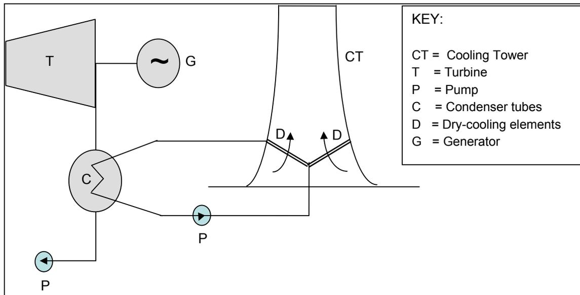
**Figure 9: Indirect dry cooling**
