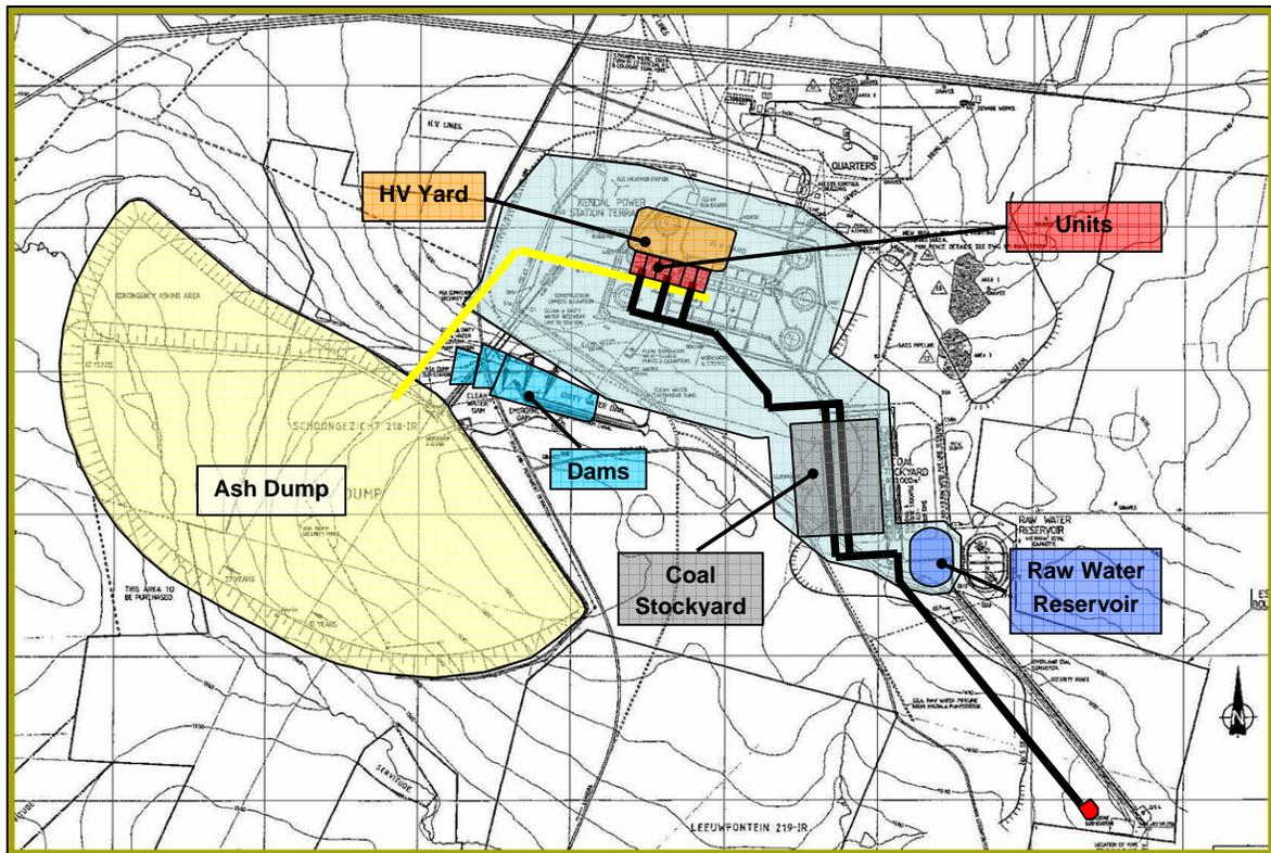
**Figure 7: Typical power station layout**
