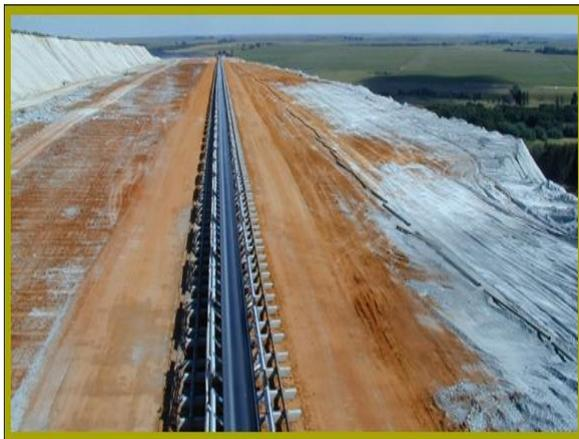
**Photo 7:** A conveyor belt on an existing ash dump.
