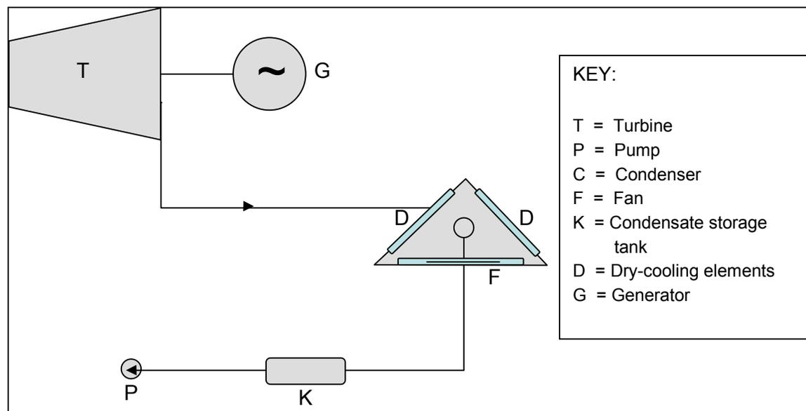
**Figure 8: Direct dry cooling**
