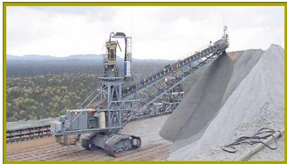
**Photo 8:** A stacker stacking ash, which will be spread out later.
