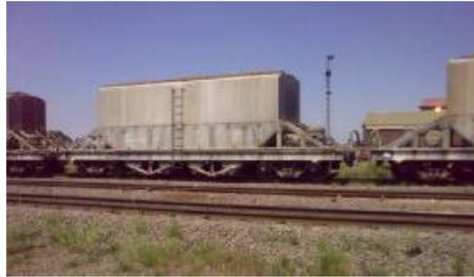
FIGURE 4-1: EXAMPLE OF A BOTTOM DISCHARGE WAGON.
