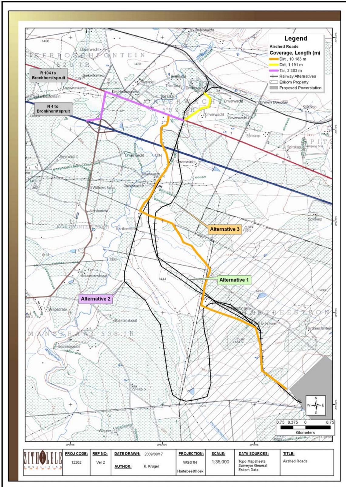
**Figure 1-1: Three proposed alternative railway corridor routes considered for the current assessment.**
