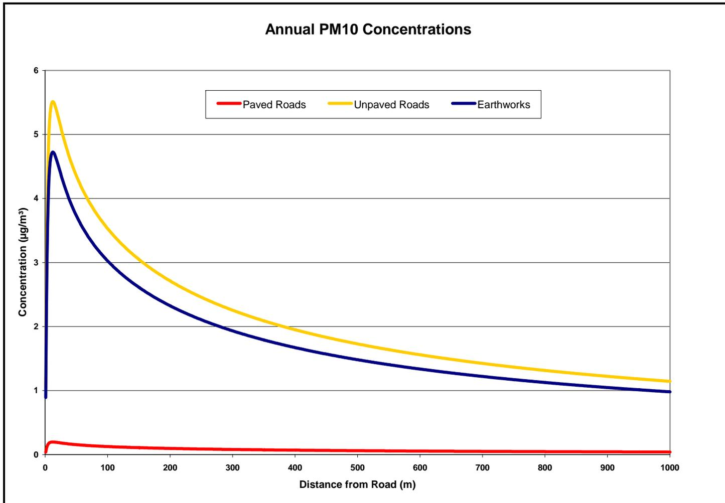
**Figure 4-4: Annual average PM10 concentrations due to vehicle entrainment on paved and unpaved road surfaces as well as earthworks for proposed construction operations.**
