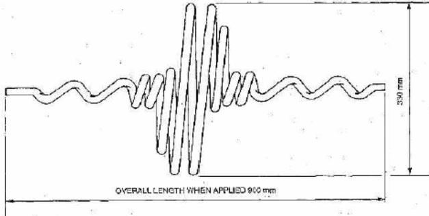
**Material Used:** Manufactured from rigid solid high impact polyvinyl chloride, possessing excellent chemical and strength properties and which will retain good physical characteristics within the range of extreme temperatures. Outdoor aging tests indicate that the material does not deteriorate in function or appearance from the effects of severe weather conditions. Industrial fumes and salt water cannot seriously degrade the properties of rigid PVC.
