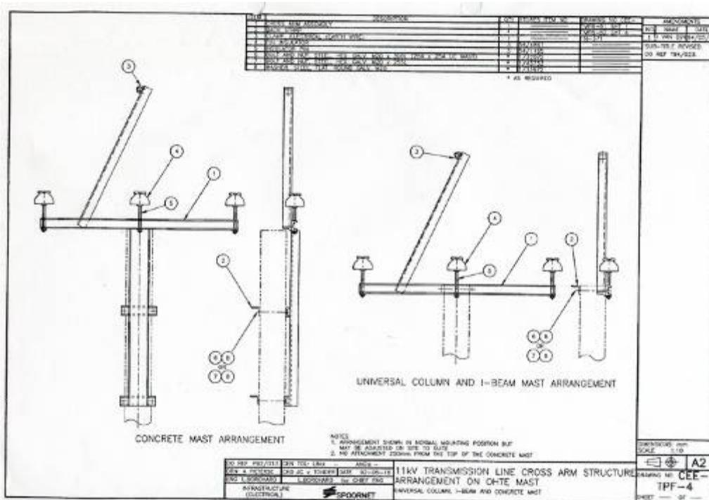
Figure 5: 11kV transmission line cross-arm structure on OHTE mast
