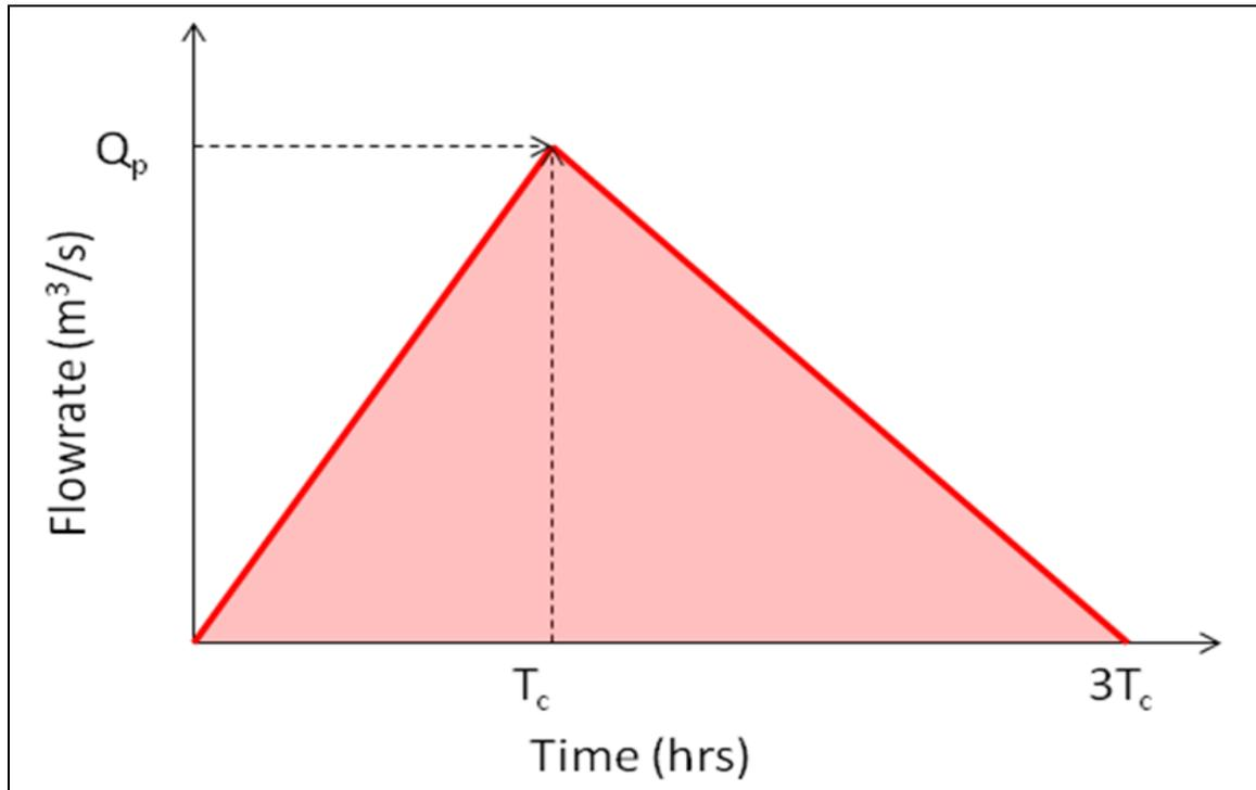
Figure 3: Triangular Hydrograph used to calculate the storm volume
