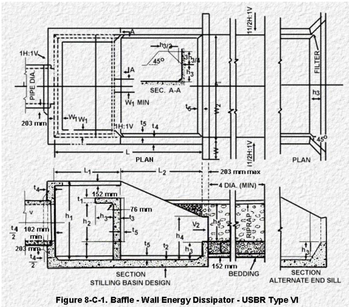
**Figure 8-C-1. Baffle - Wall Energy Dissipator - USBR Type VI**
